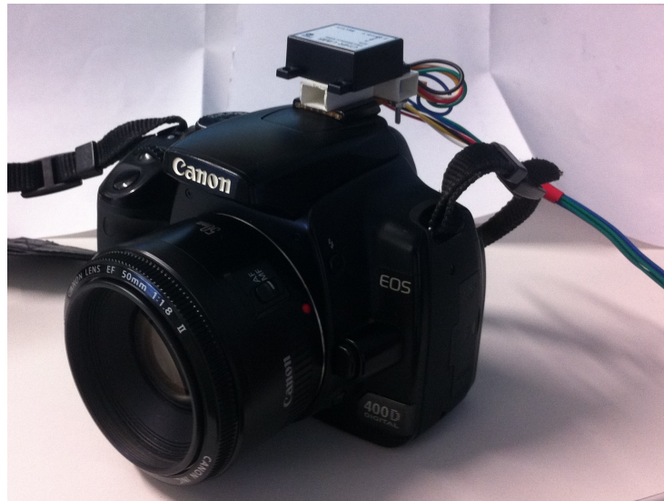
Figure 6.1: The Camera with an Orientation Sensor Mounted on the 'Hot-Shoe'
