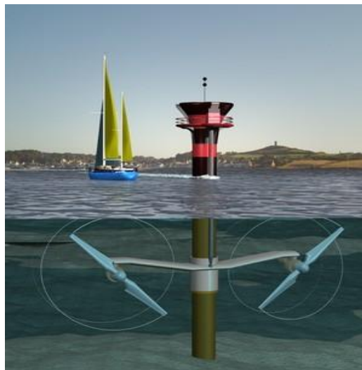
Figure 3.10 SeaGen twin horizontal axis turbines on fixed support tower
