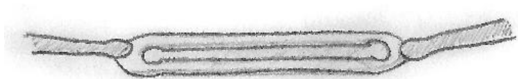
Fig. 2. An illustration of the drawing method of glass bead manufacture. A tube of molten glass is drawn out, before individual beads are produced and severed from it.
