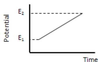
Figure 3.2 – The potential model for linear sweep voltammetry.
