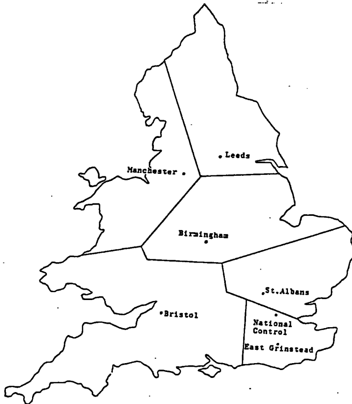
FIGURE 1.2 LOCATION OF THE GRID CONTROL CENTRES
