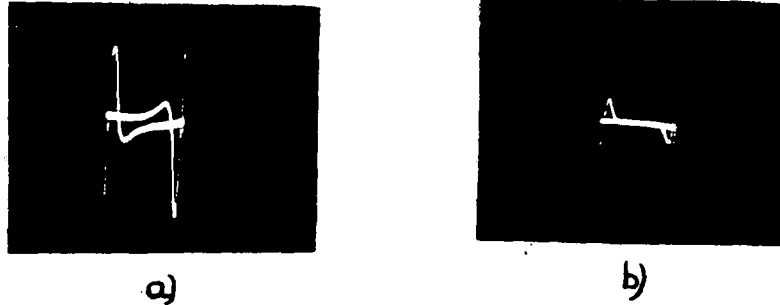
Fig. 53). Bridge output waveforms for:- a) Soda glass, b) Hysil glass.
