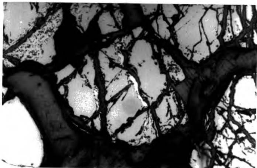
Plate 35 "Ferritchromit" zones developed along grain boundaries and cracks in chromite (Reflected light, X80).
