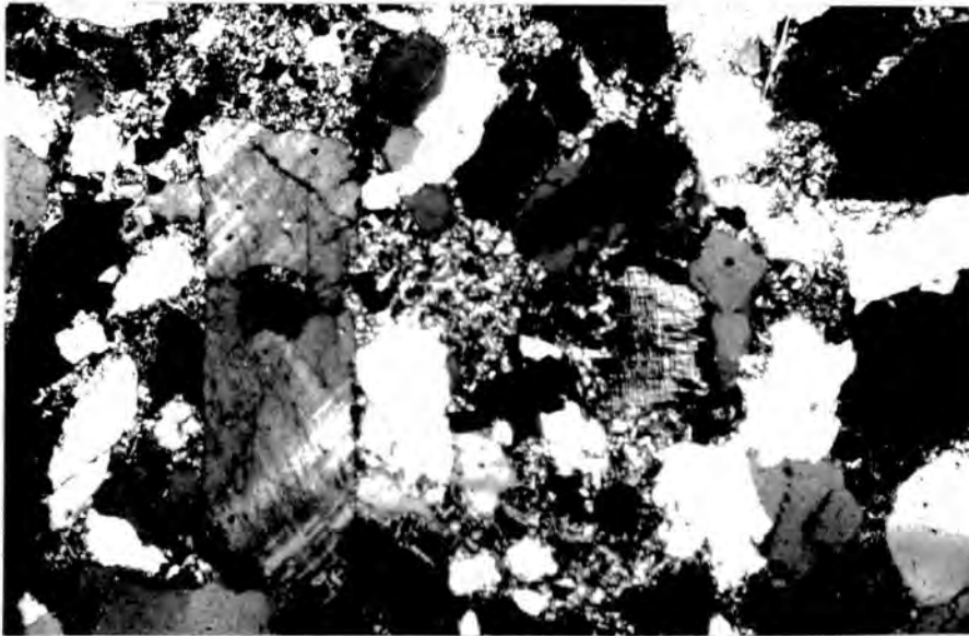
PLATE 29. Microcrystalline silica cement in sub- arkose, Low Grit Sill. (x 30)
