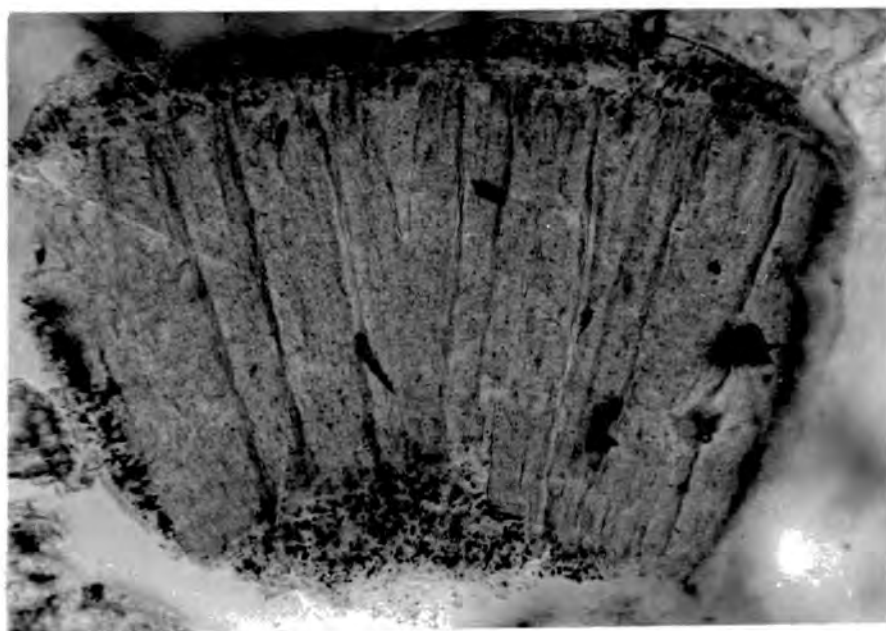
PLATE 44. "Accordion-structure" in authigenic chamosite. (x 400)
