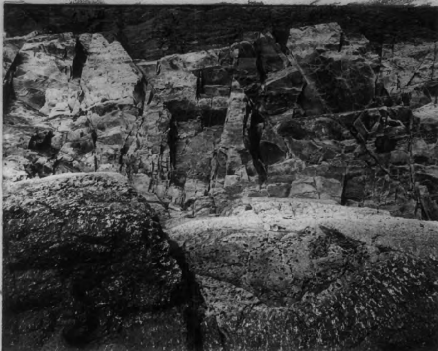
Plate 5.11 COMPLEMENTARY PRIMARY WRENCH-JOINTS North side of Freshwater East (3003) Steeply dipping wrench-joints lie symmetrically about the traces of the rotation joints (plunging gently left) on the vertical bedding planes of Lower Old Red Sandstone marls.
