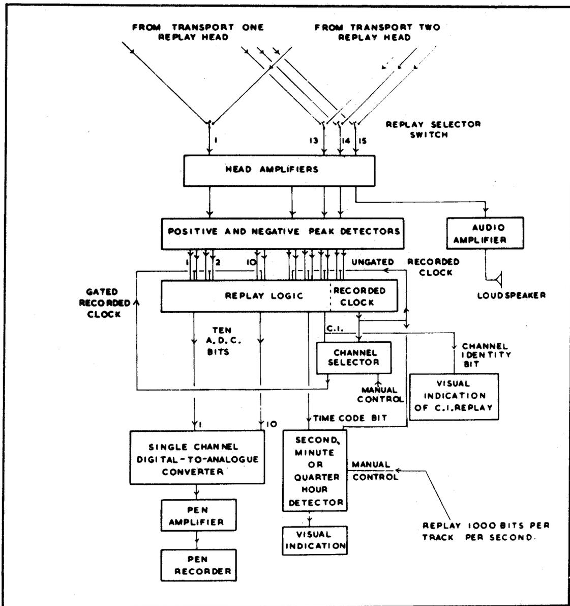
Fig.11. Schematic diagrams of seismic data processing system (after Lucas 1966).
