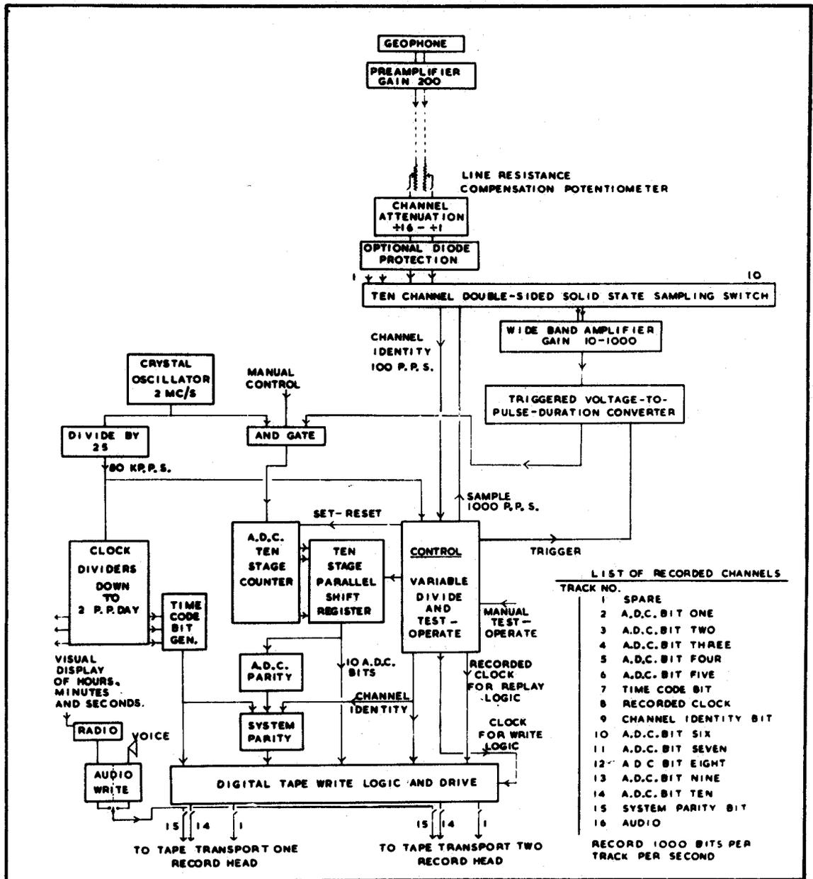
Fig.10. Schematic diagrams of seismic data processing system (after Lucas 1966).
