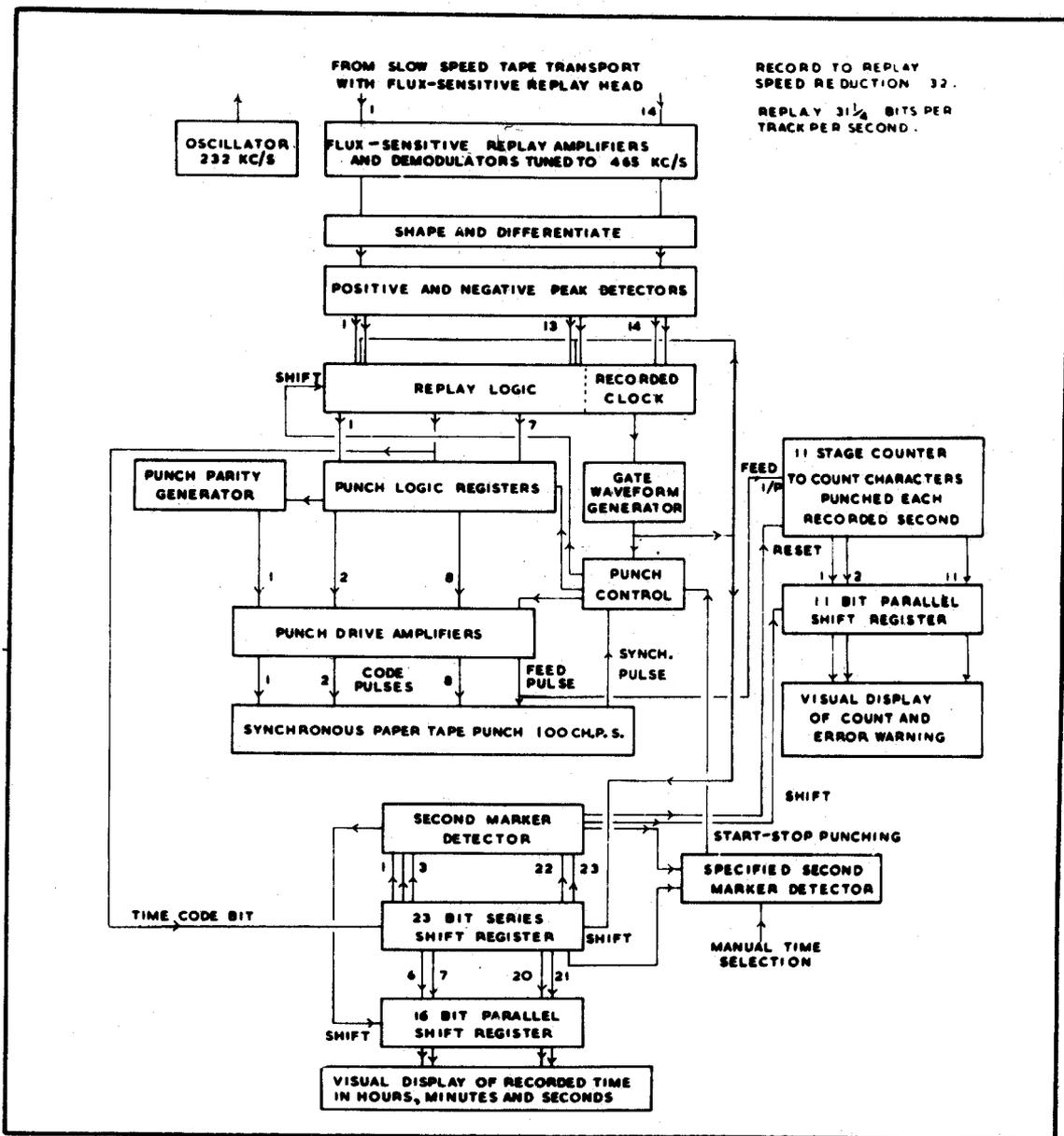
Fig.14. Schematic diagrams of seismic data processing system (after Lucas 1966).
