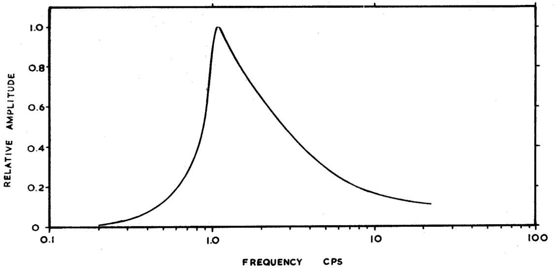
Fig.28. Frequency responses of the recording systems at the Scilly Isles station (above) and at the Carnmenellis and Bodmin Moor stations (below).
