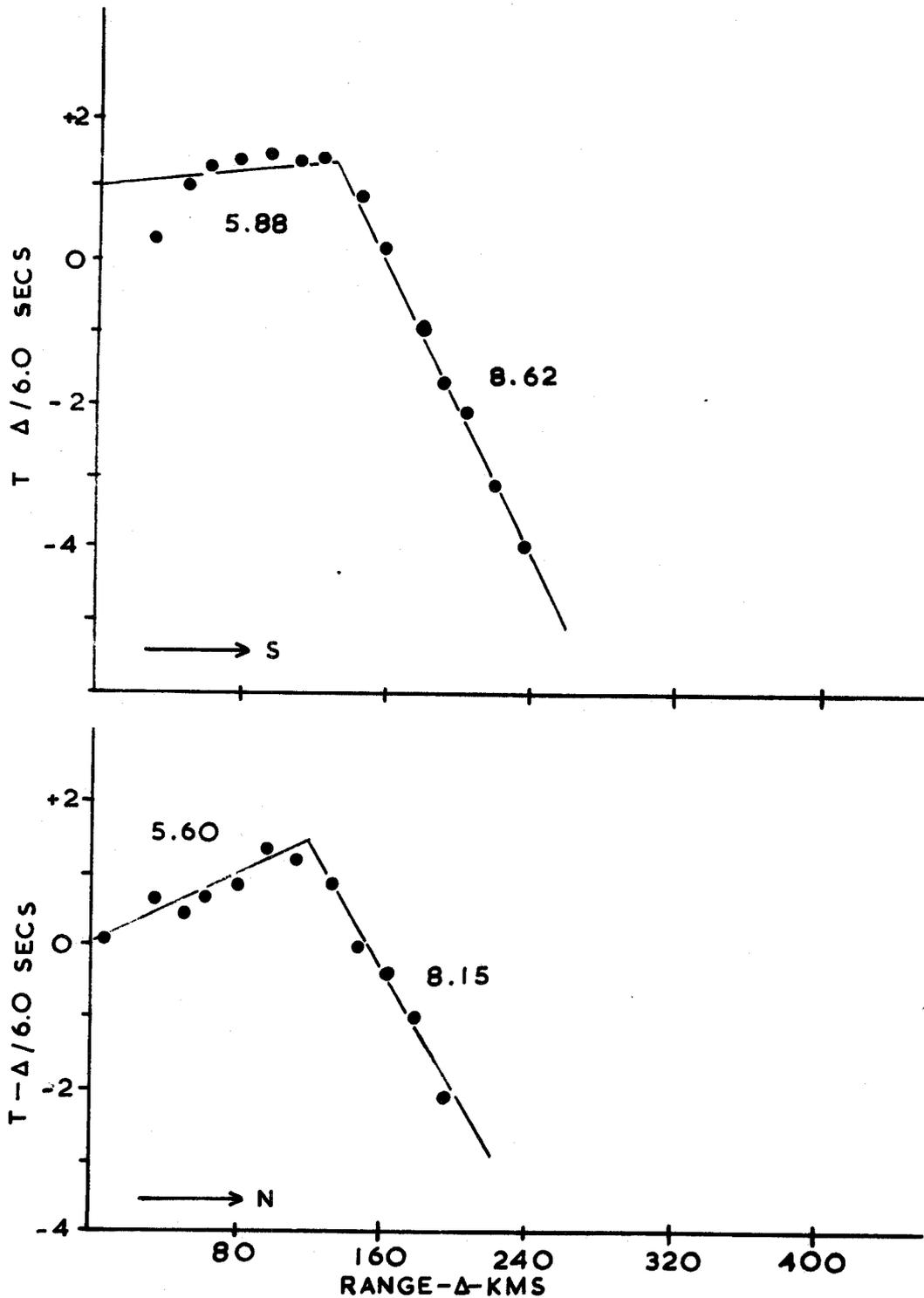
Fig.21. First arrival travel time graphs for the Waterford station (above) and the Land's End station for the line 2 shots (below).
