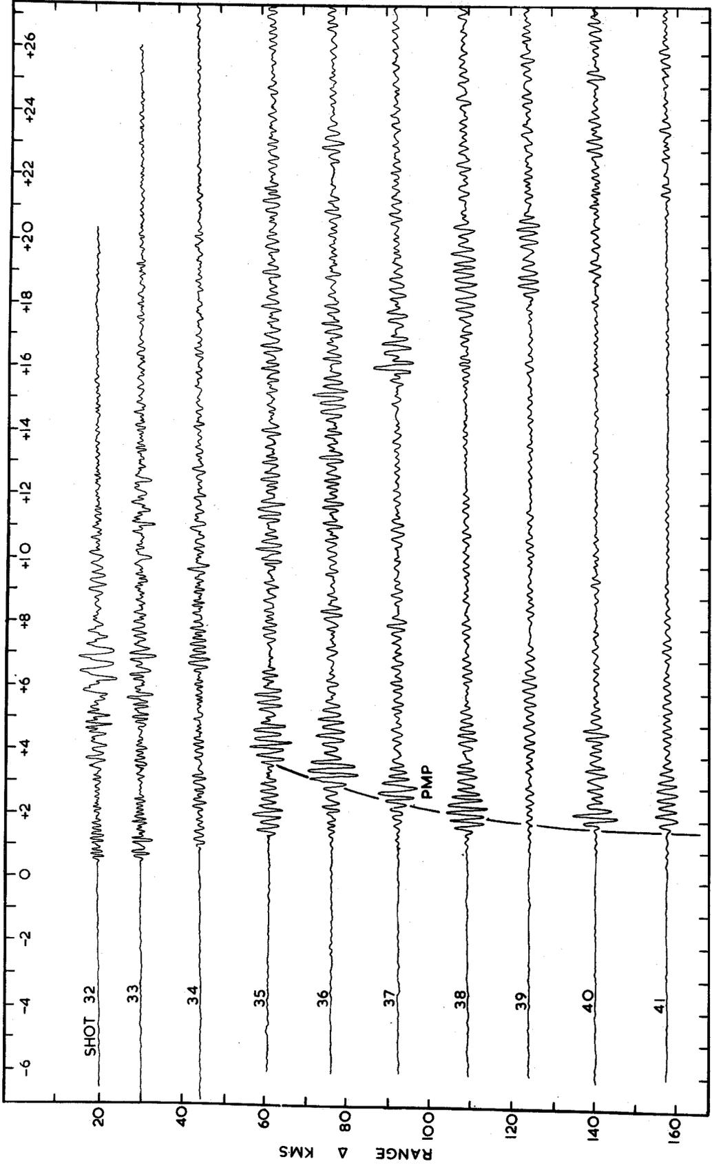
Fig.38. The stacked record of the line 3 shots at the French stations.
