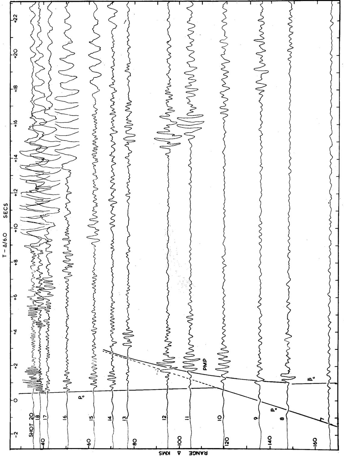
Fig.33. The stacked record of the line 1 shots at the Bodmin Moor station.
