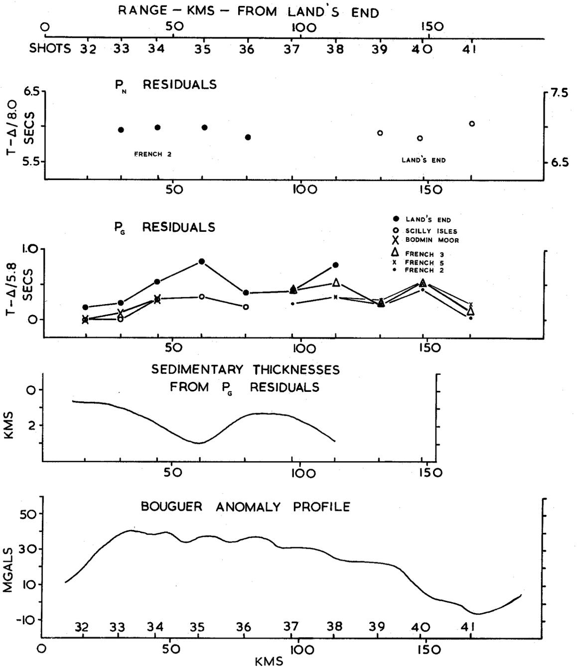
Fig.25. Residual data from line 3.
