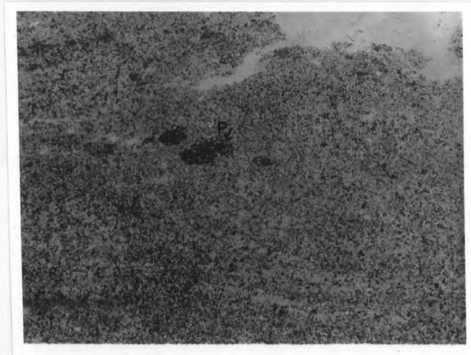
Fig. 4.4. Type 2 sandstone, T.248, showing argillaceous matrix and pyrite, P. Ordinary transmitted light X 10
