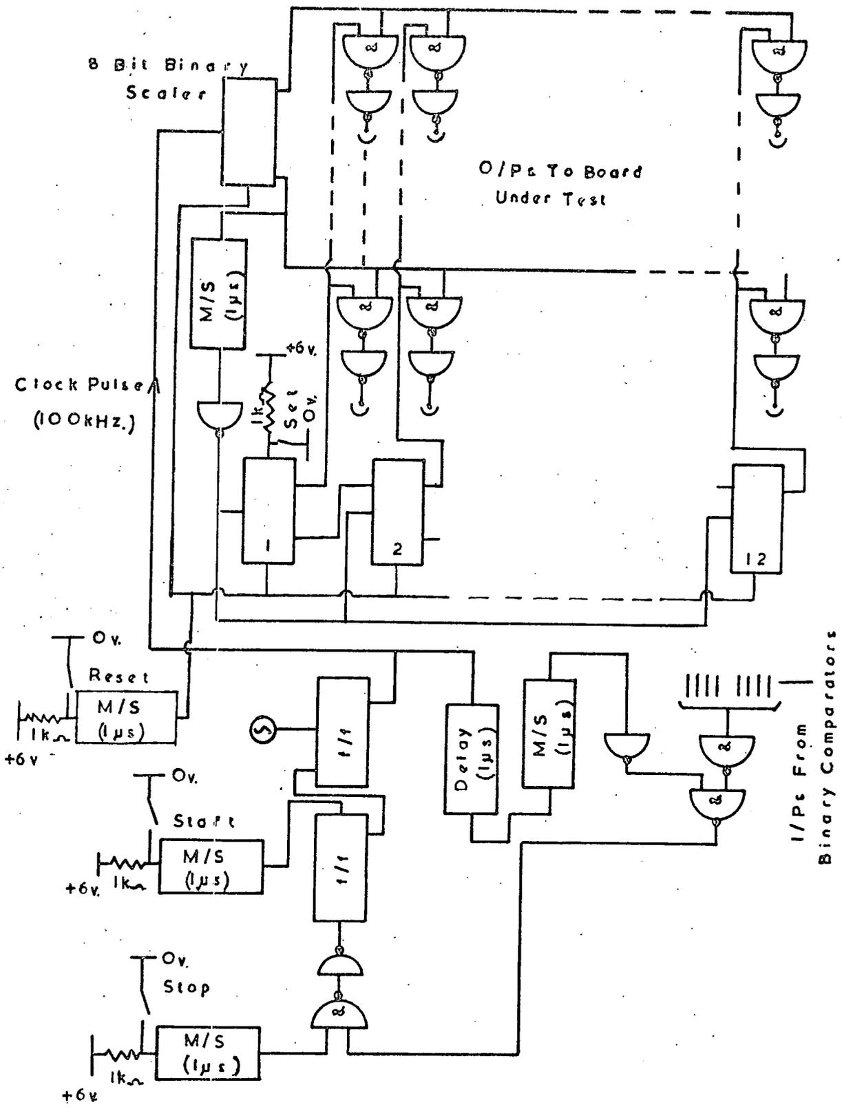
Figure 6.13 The Circuit for the Mixer Board Tester.
