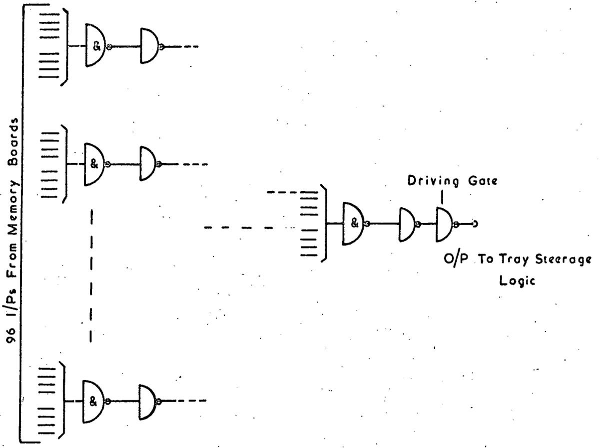
Figure 6.8 The Circuit for the Scan Control Board.
