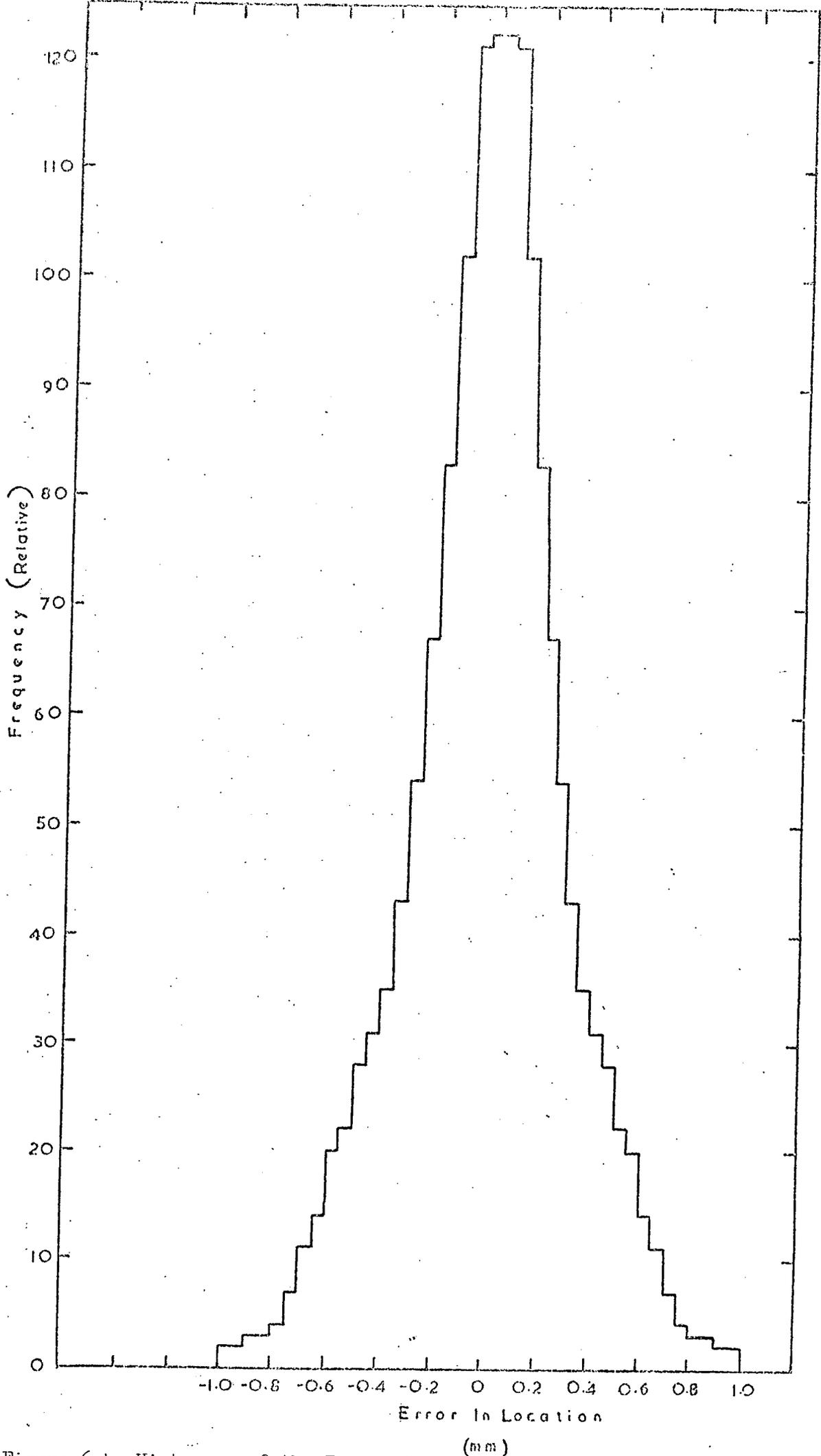
Figure 6.4 Histogram of the Errors in Location for a Measuring Tray Tube Spacing.
