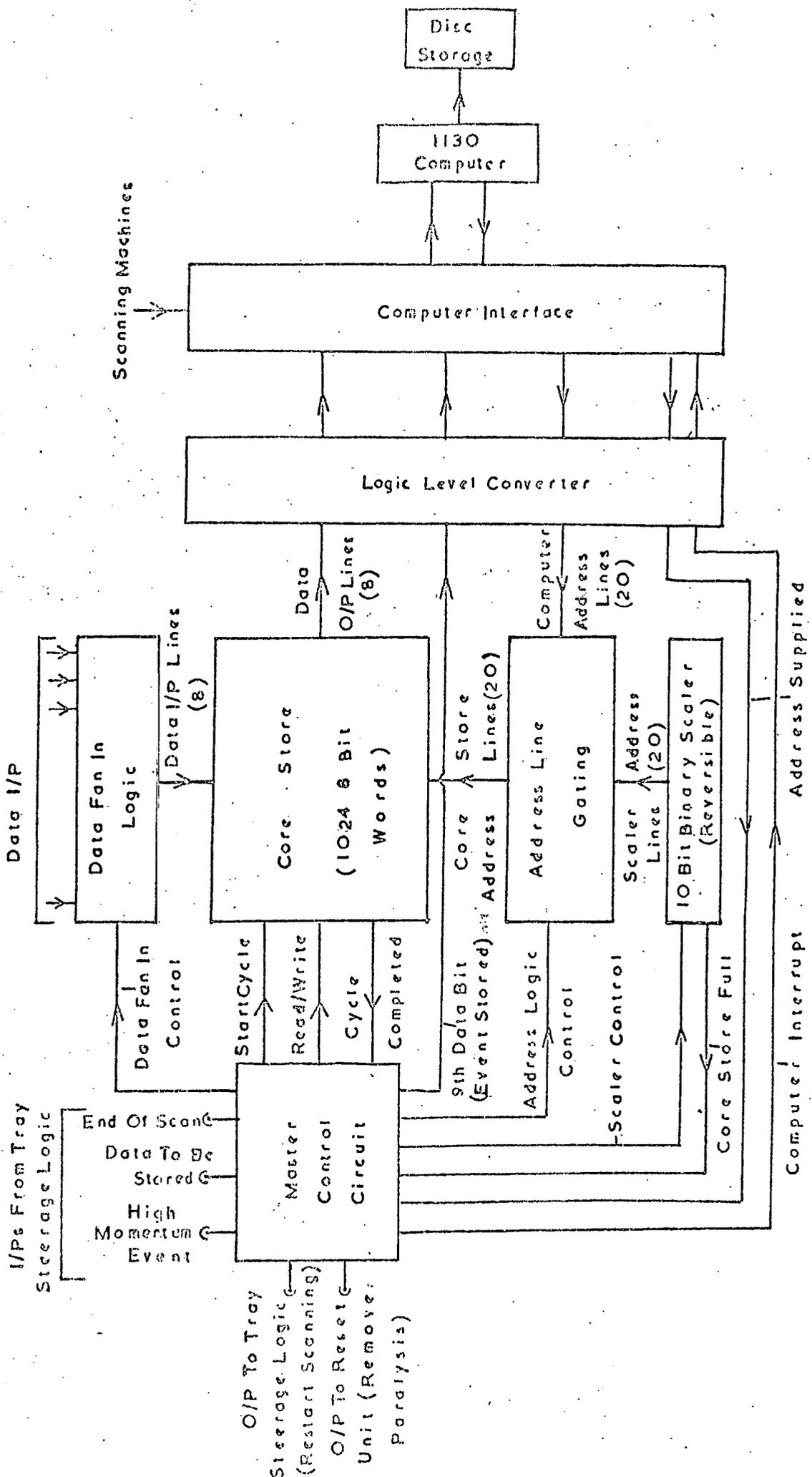
Figure 6.16 Block Diagram of the Core Store Logic.
