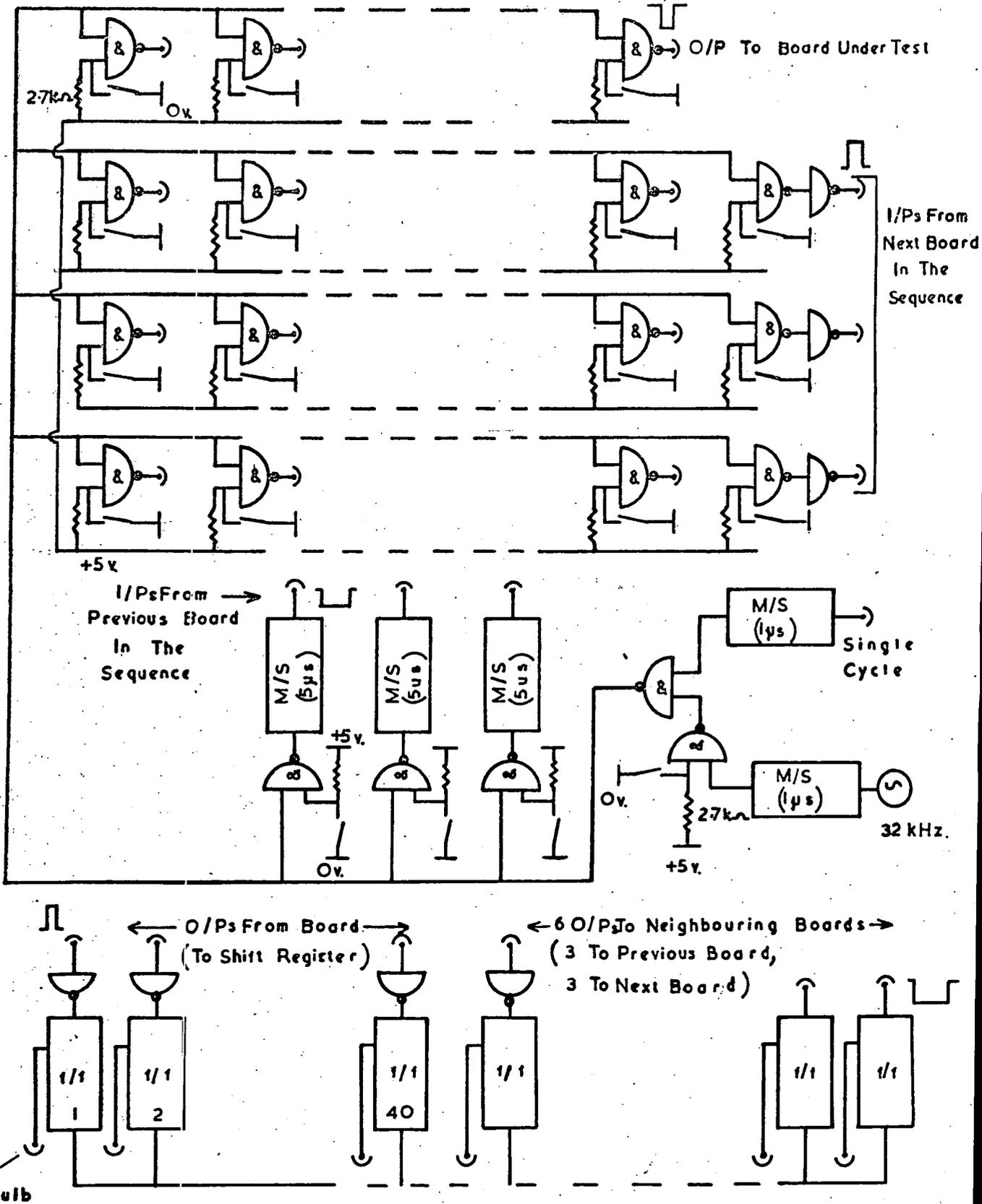
Figure 5.16 The Test Circuit for the Cell Allocation Logic Boards.
