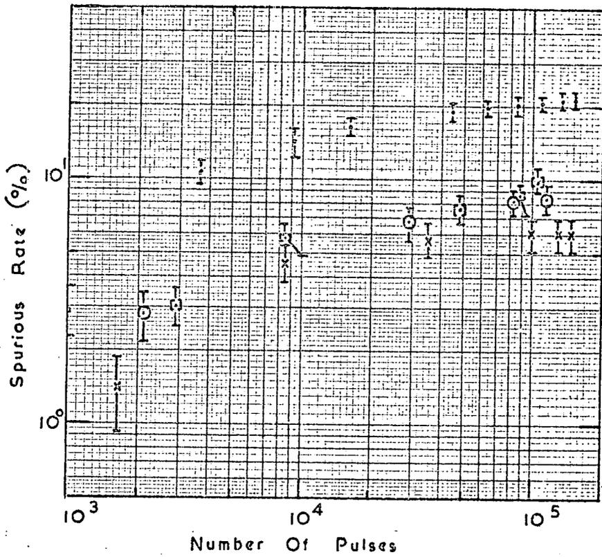
Figure B.3 Graphs of the Spurious Rate against Number of Pulses for Various Electrode Sizes.
