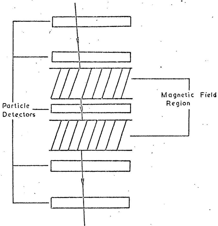
Figure 2.3 Schematic Form of a Multilayer Spectrograph.
