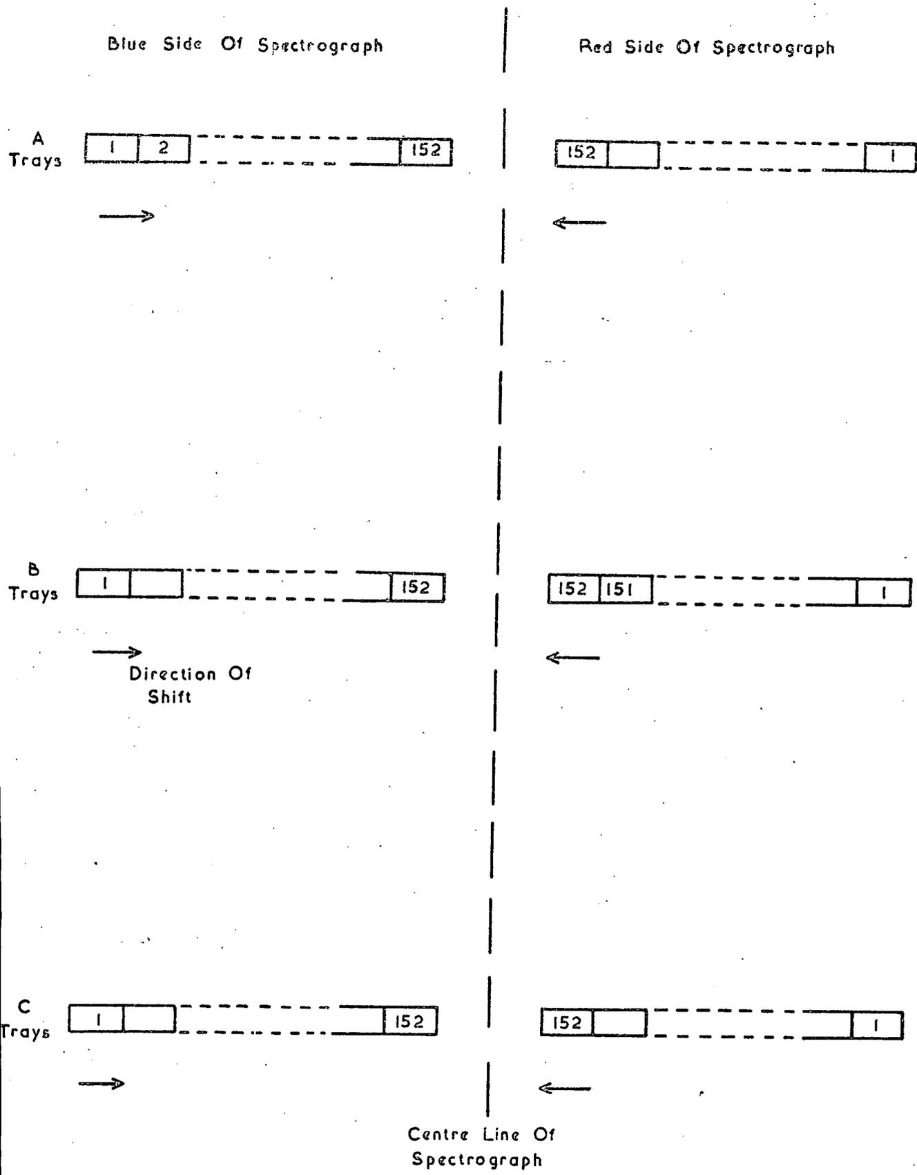
Figure 5.18 The Cell Numbering and Shift Directions in the Momentum Selector Trays.
