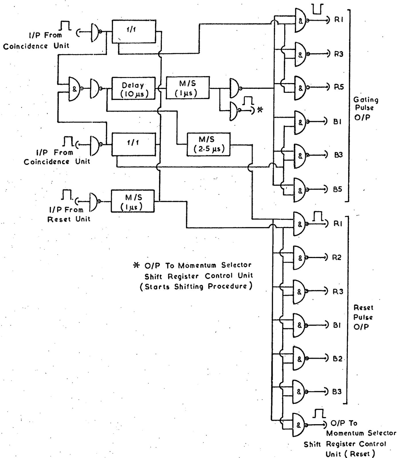
Figure 5.20 The Circuit for the Momentum Selector Control Unit.
