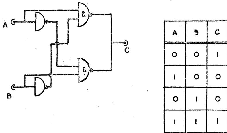
Figure A.8 The Binary Comparator Circuit.
