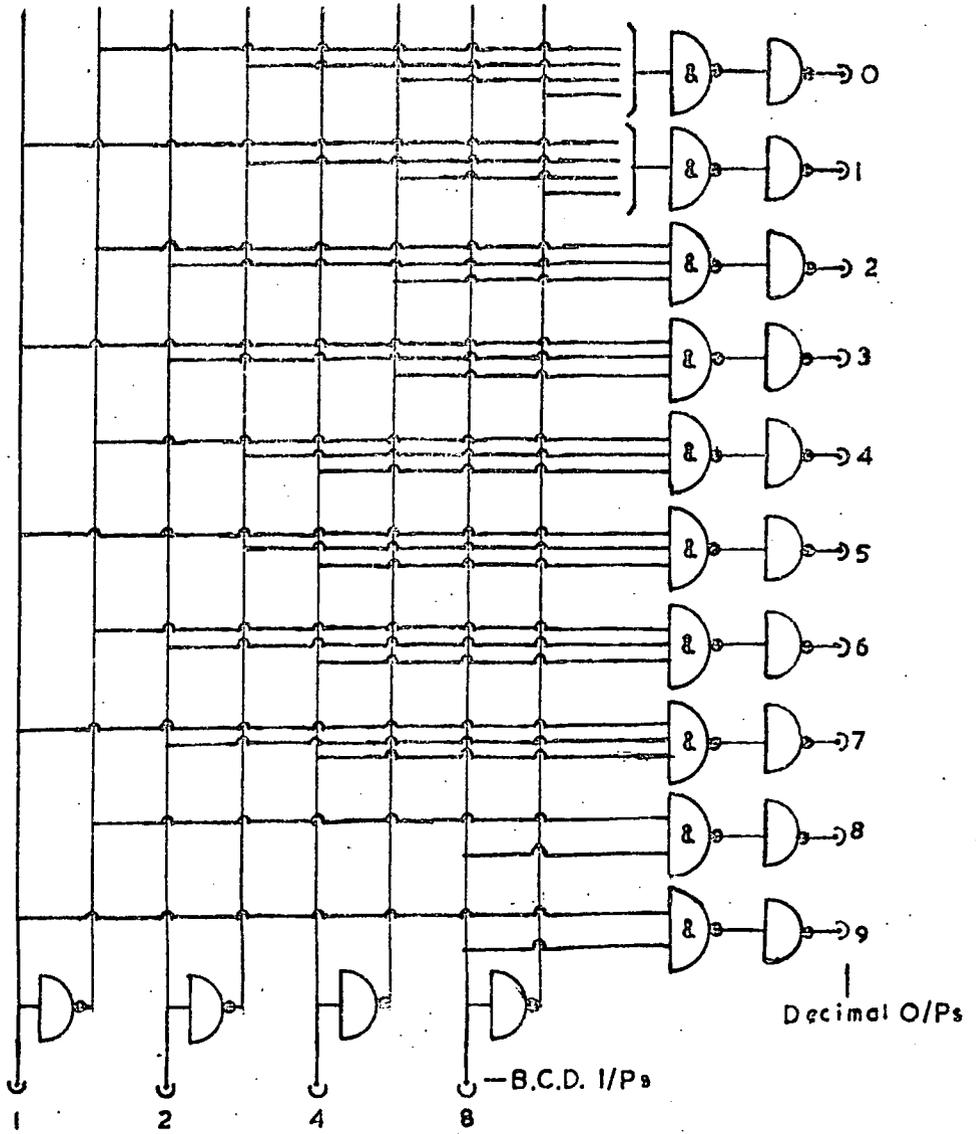
Figure A.12 The Form of the B.C.D. to Decimal Converter.
