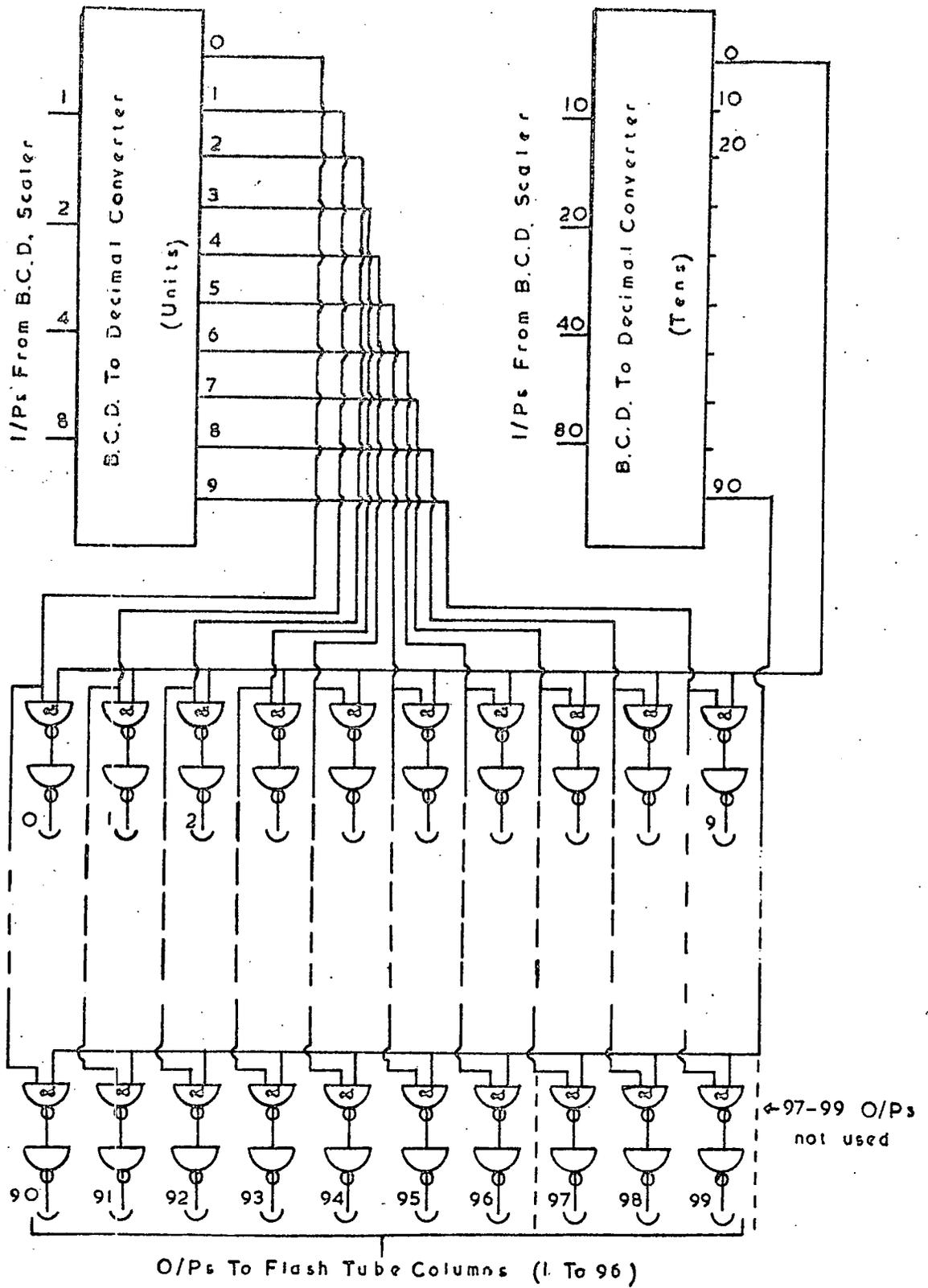
Figure 6.7 The Circuit for the Gating Logic.
