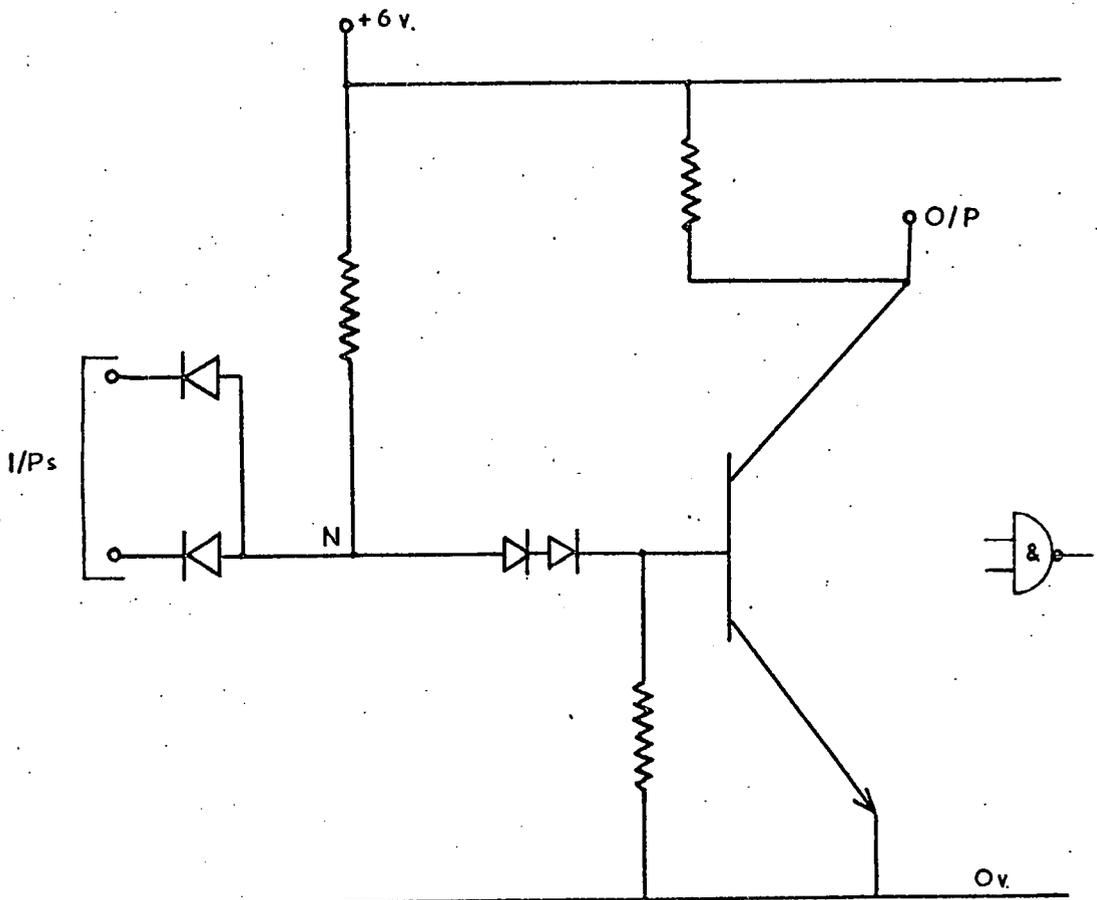
Figure A.6 Schematic Diagram of a Two Fold DTL Nand Gate
