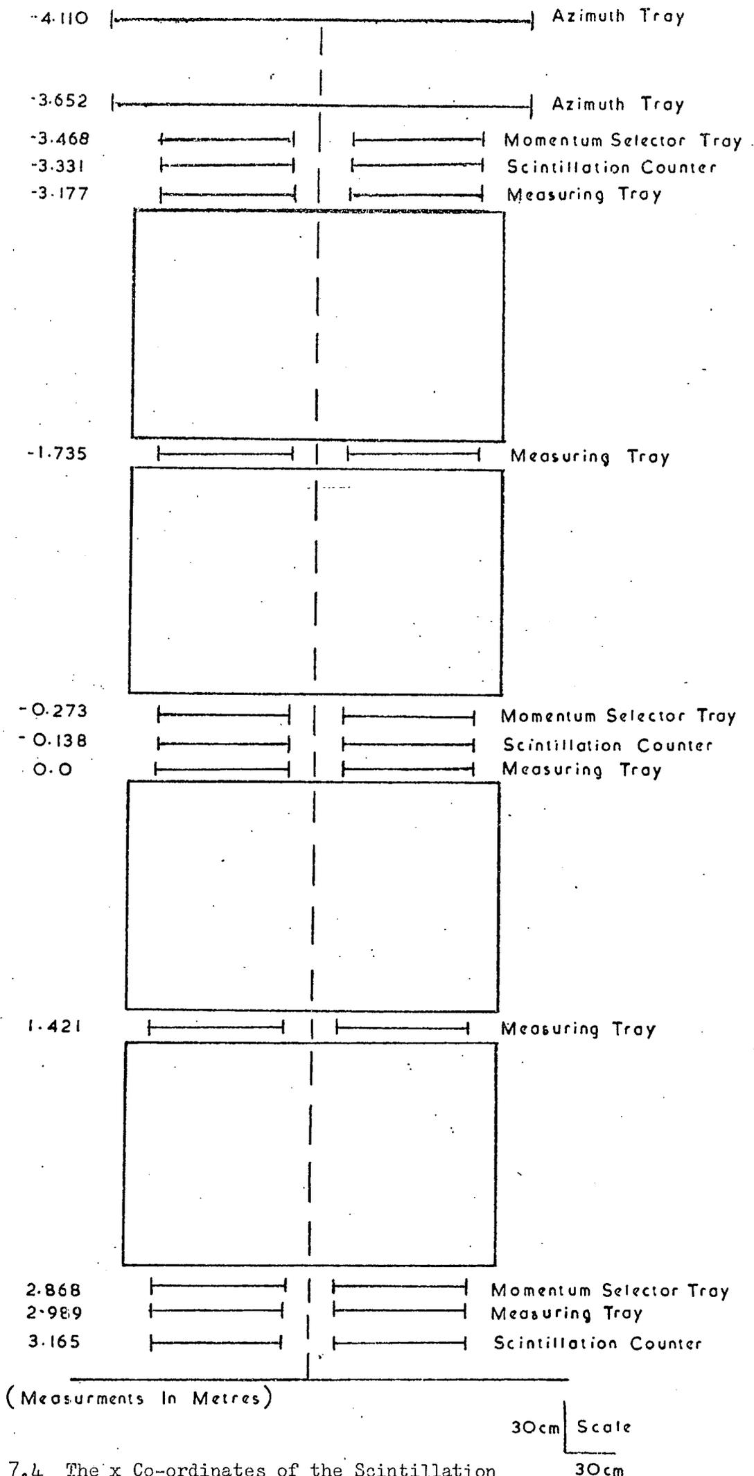
Figure 7.4 The x Co-ordinates of the Scintillation Counters and Flash Tube Trays in the Spectrograph.
