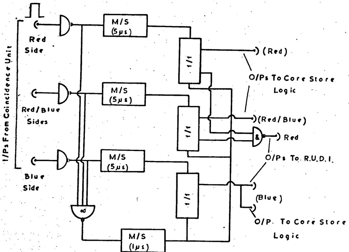
Figure 6.21 The Circuit for Digitising the Trigger Mode.
