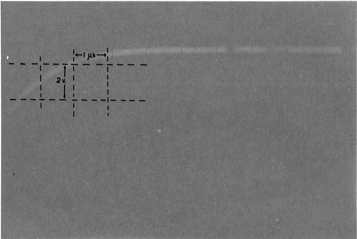
events when the output from the probe is fed directly into an oscilloscope of input impedance  $10^7$  ohm with no output resistor.
