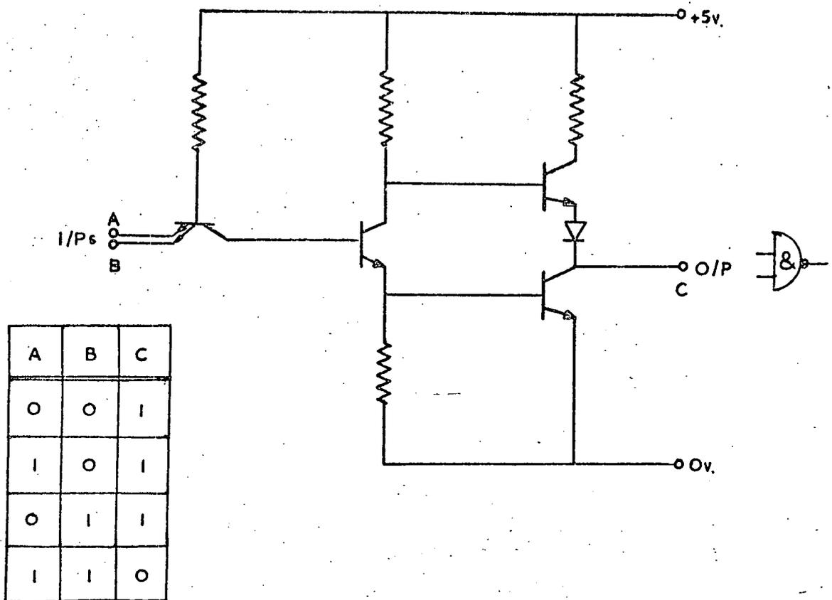
Figure A.1 Schematic Diagram of a Two Fold TTL Nand Gate.
