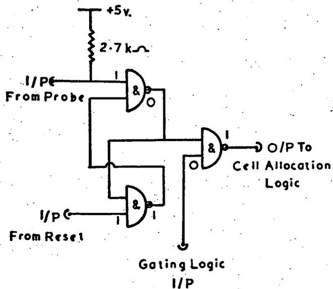
Figure 5.12 The Electronic Memory and Gating System used with each Flash Tube Probe.
