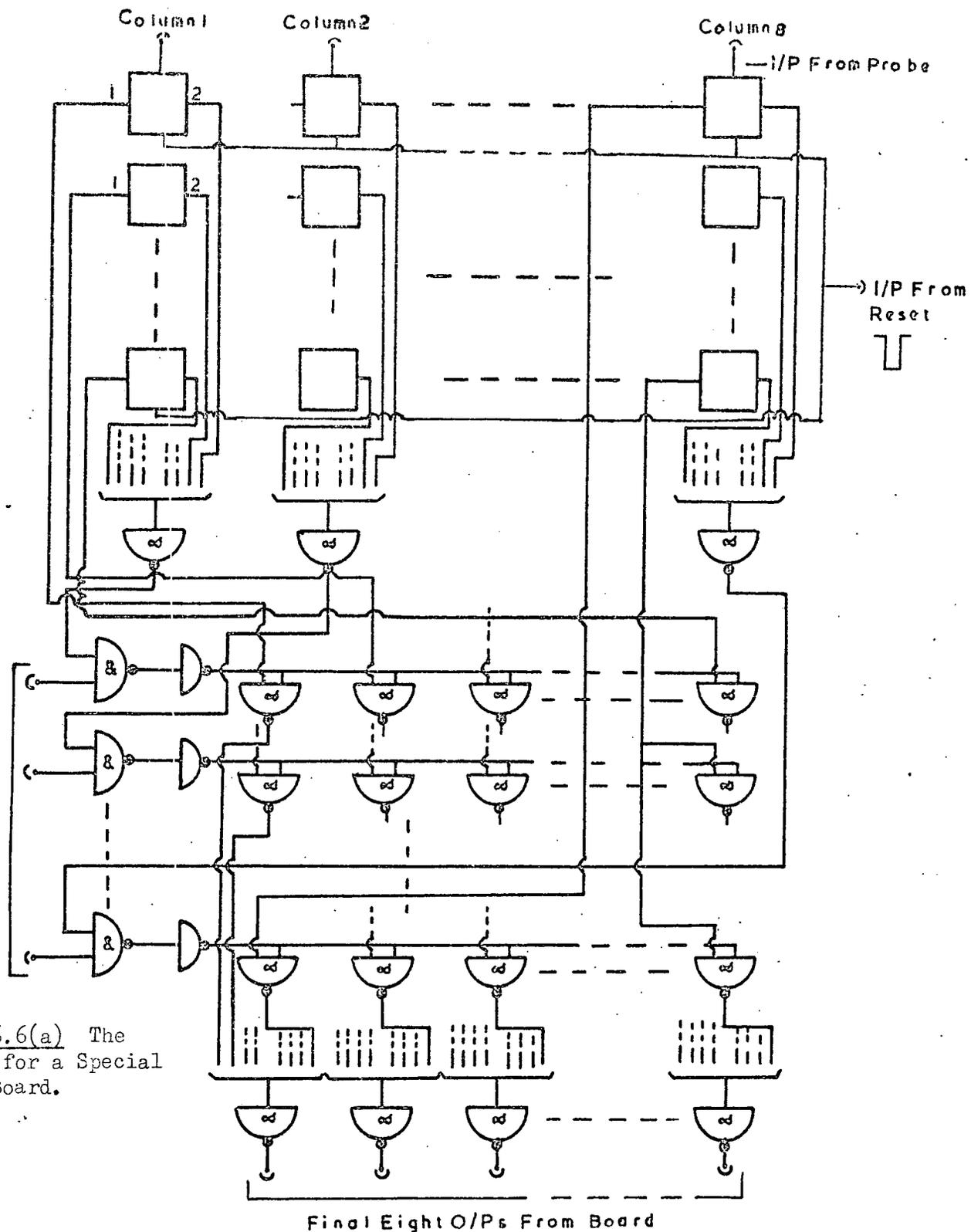
Figure 6.6(a) The Circuit for a Special Memory Board.
