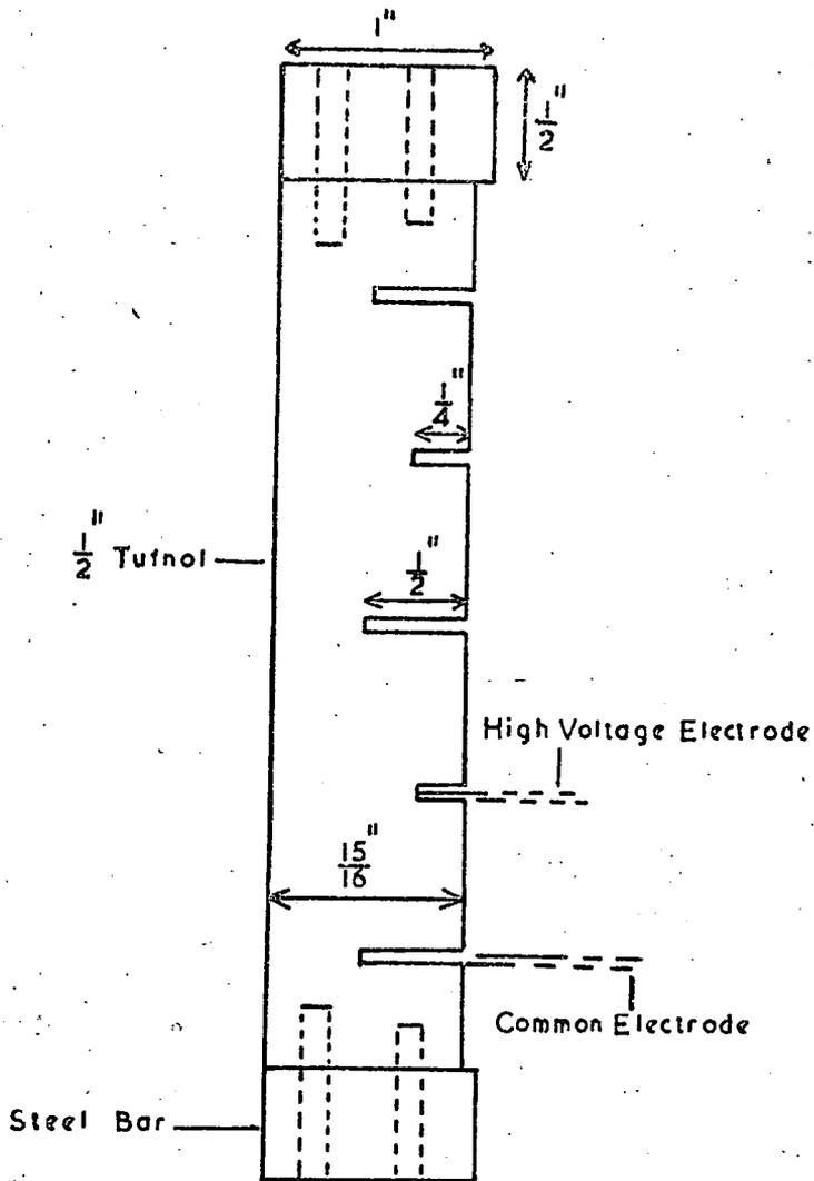
Figure 5.4 Cross-sectional View of a Tufnol Electrode Support.
