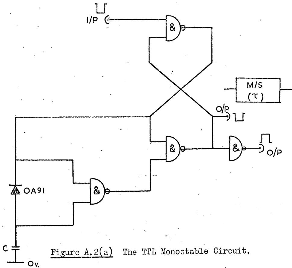
Figure A.2(a) The TTL Monostable Circuit.
