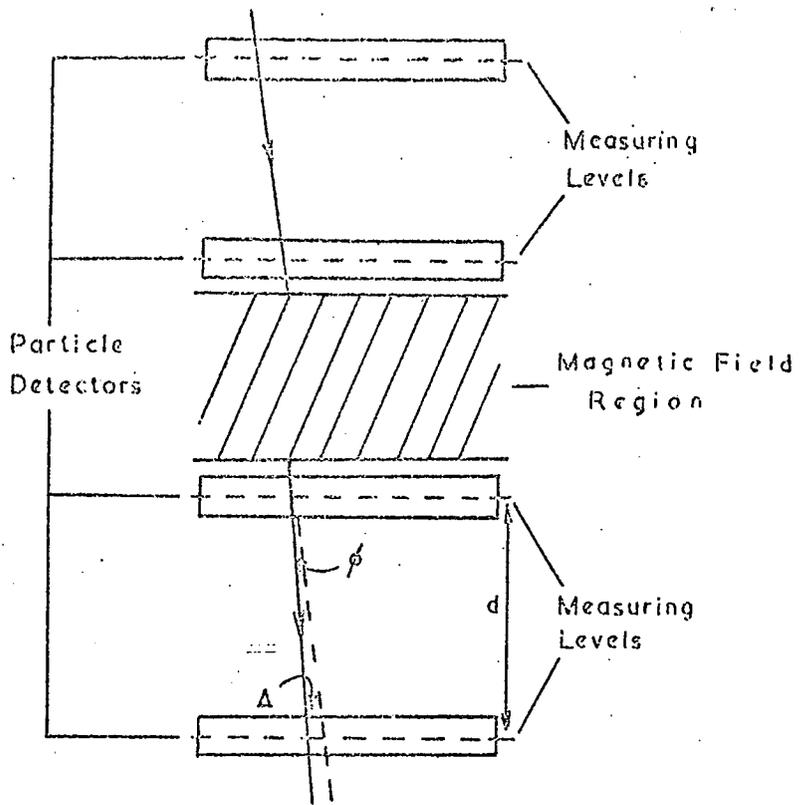
Figure 2.2 Schematic Form of a Conventional Spectrograph.
