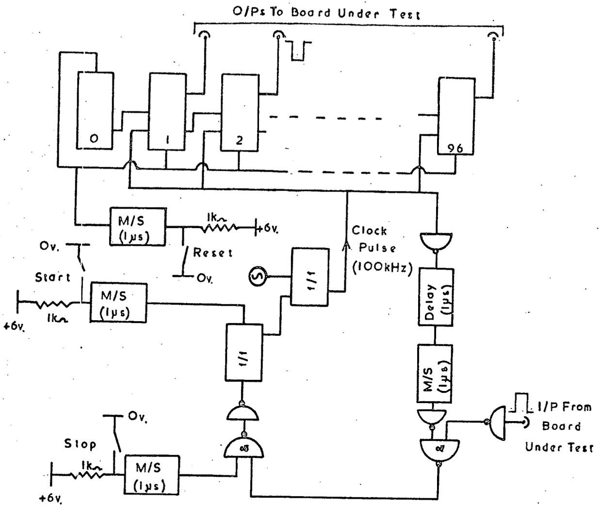
Figure 6.12 The Circuit for the Scan Control Board Tester.
