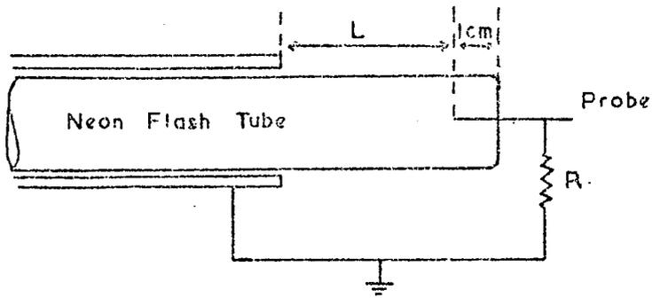
Figure 4.8(a) The Experimental Arrangement for Investigating the Voltage Pulse inside the Flash Tube.
