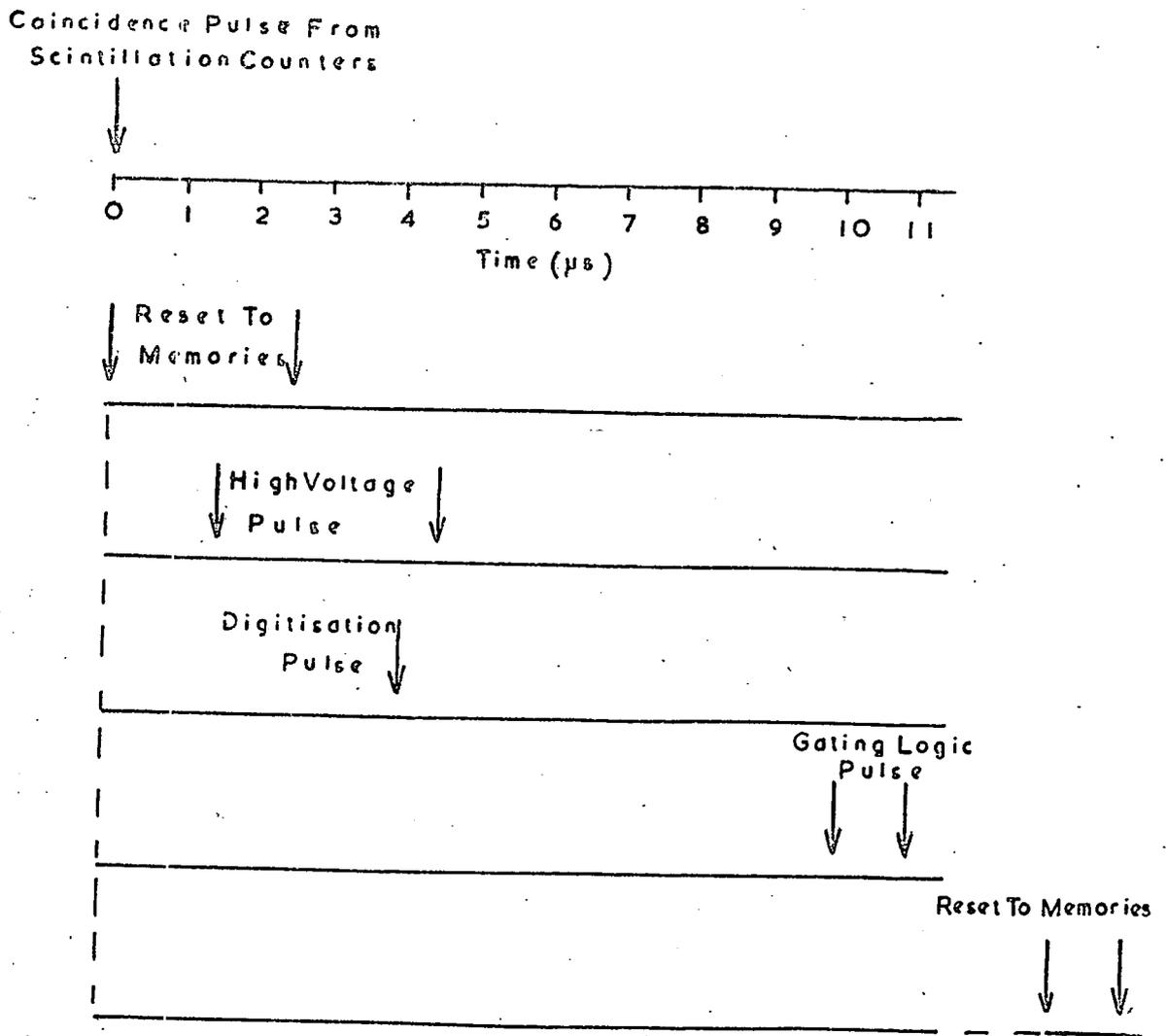
Figure 5.21 The Sequence of Pulses in the Momentum Selector System when a coincidence pulse is obtained from the Scintillation Counters.
