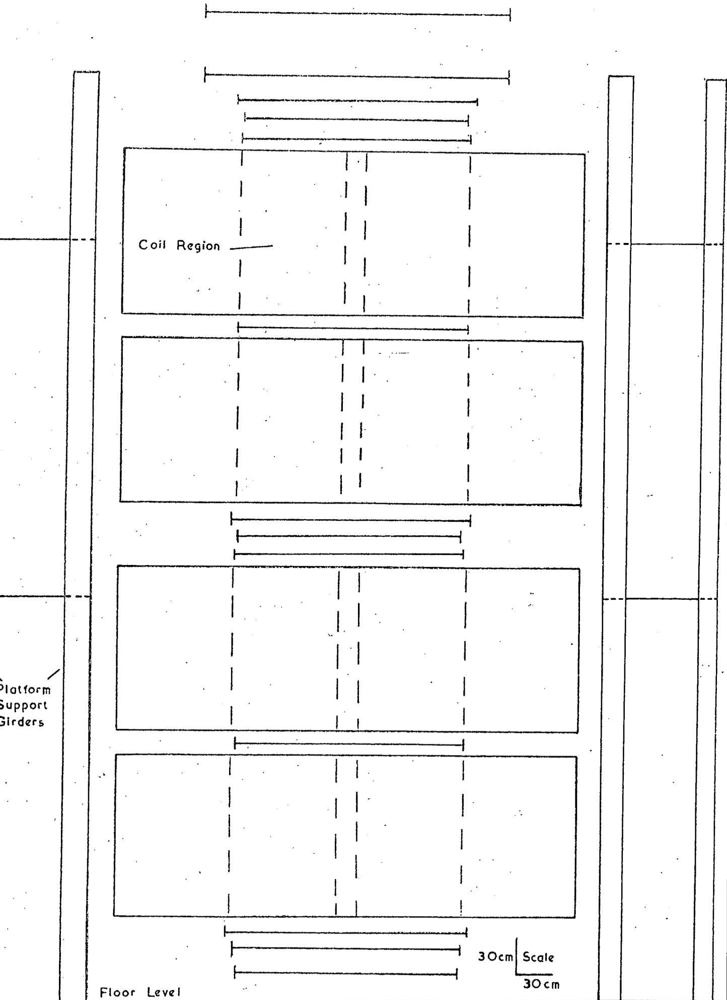
Figure 3.2 M.A.R.S. : Side View of the Spectrograph.
