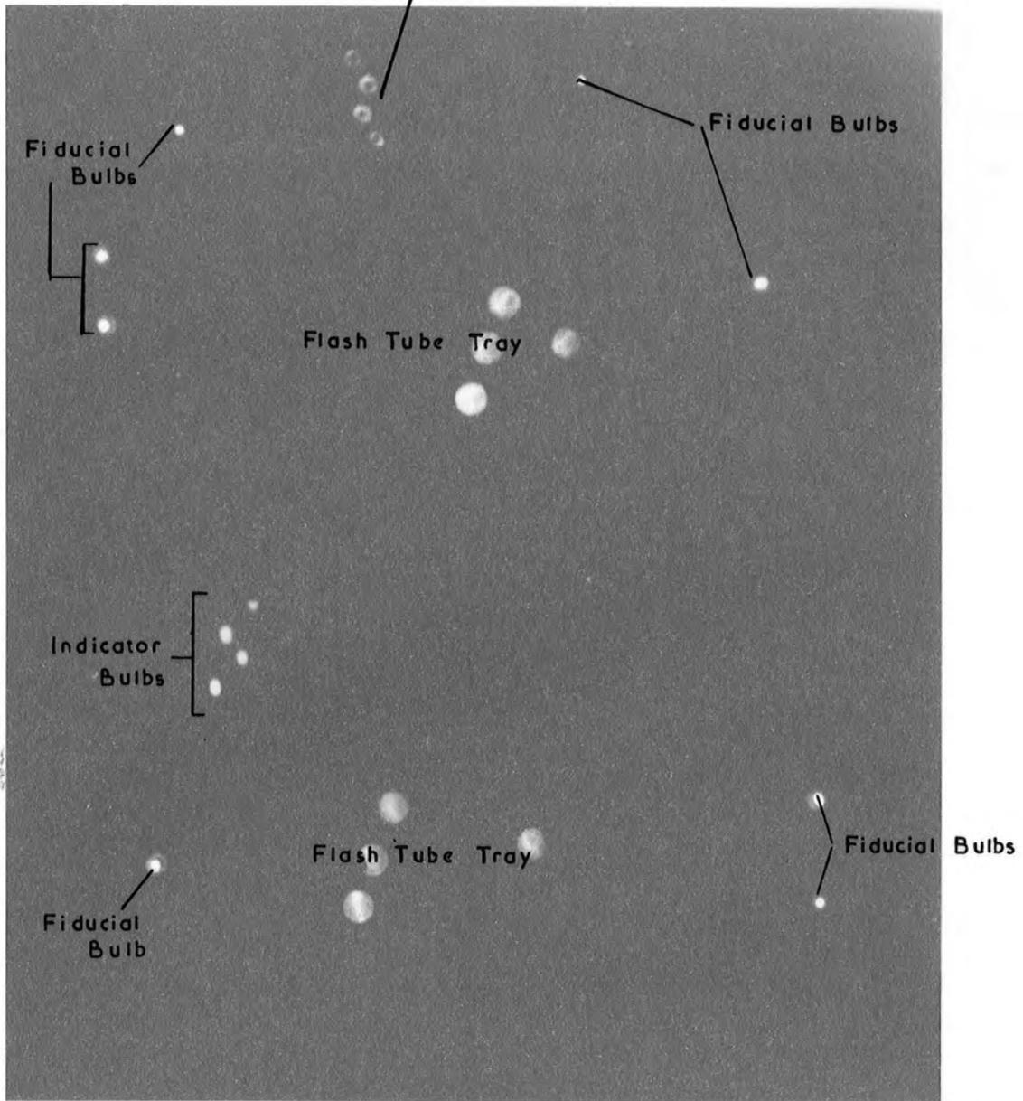
were placed above and below the flash tube tray and the high voltage pulse was applied to the tray when a two fold coincidence pulse was obtained from the scintillation counters.
