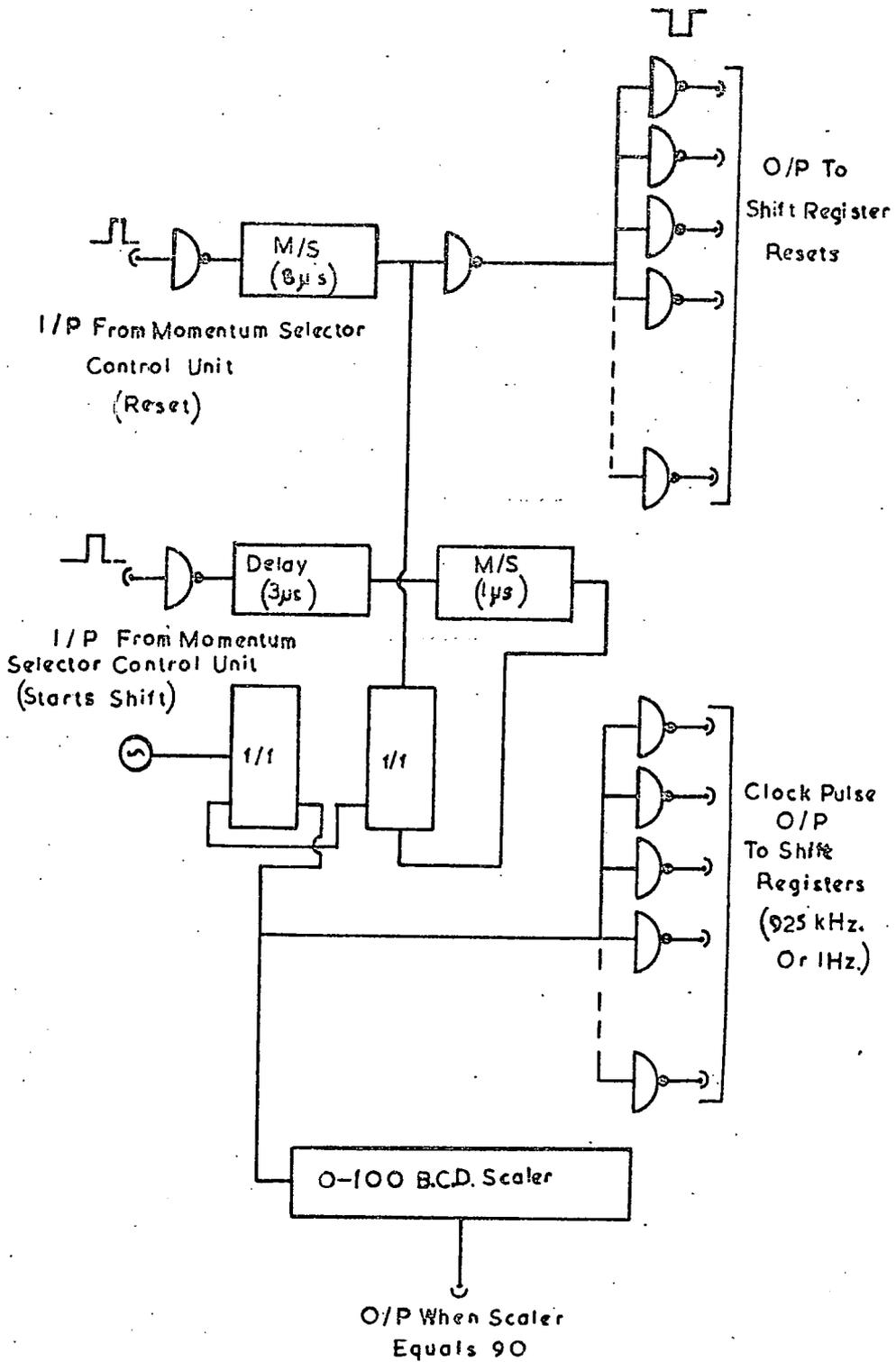
Figure 5.22 The Circuit for the Momentum Selector Shift Register Control Unit.
