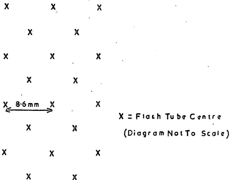
Figure 6.3(b) The Flash Tube Pattern used to obtain the Graph of Figure 6.3(a).
