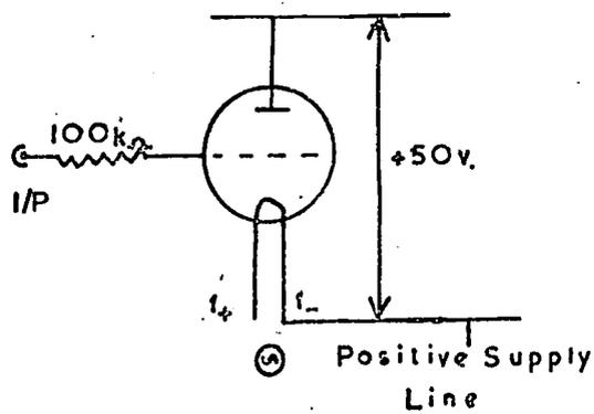
Figure A.13 Schematic Diagram of the Indicator Bulb Type DM160.
