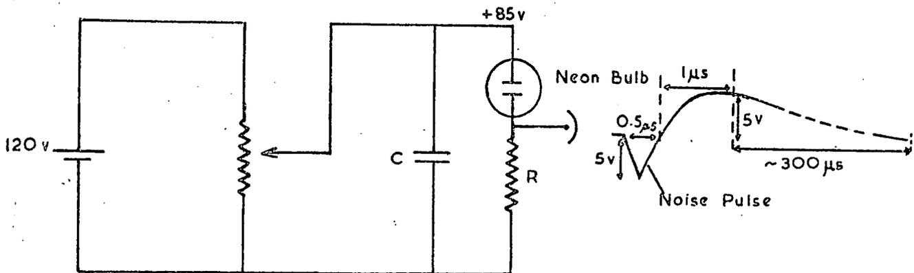
Figure 4.2 The Circuit Used with the Neon Bulb and the Output Pulse obtained with  $R = 3.3\text{k}\Omega$  and  $C = 0.01\mu\text{f}$ .
