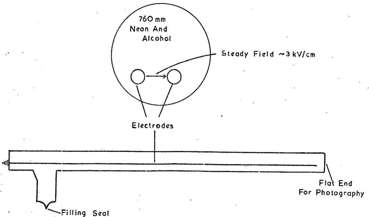
Figure 4.20 The Spark Tube Used by Bacon and Nash (1965)
