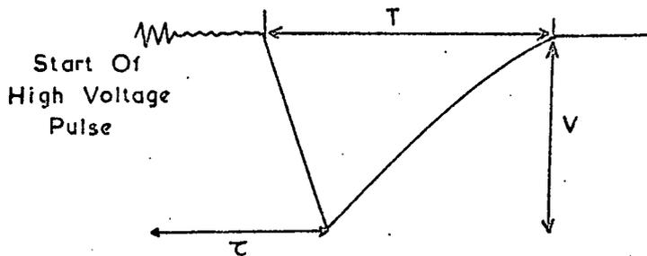
Figure 4.8(b) Form of Pulse obtained for an Applied Negative High Voltage Pulse and the Measured Parameters of the Pulse.
