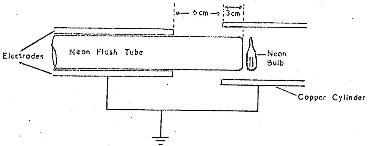
Figure 4.1 The Experimental Arrangement for the Preliminary Investigation.
