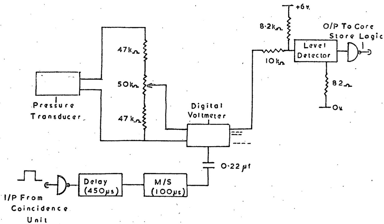
Figure 6.22 The Circuit for Digitising the Atmospheric Pressure.
