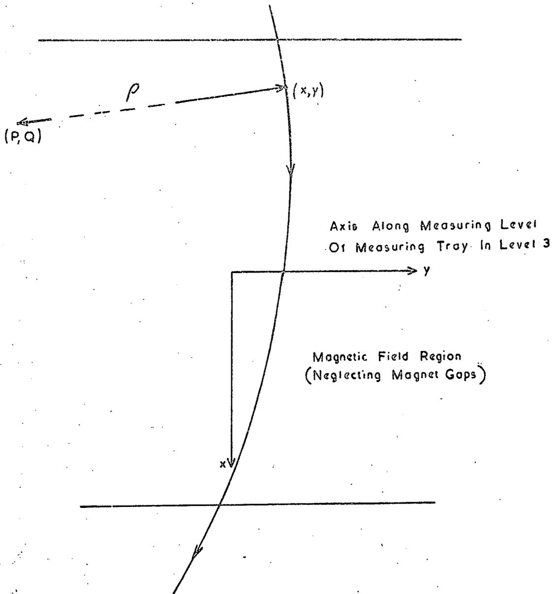
Figure 7.3 The Passage of a Singly Charged Particle Passing Through One Side of the Spectrograph with Cartesian Axes as shown.
