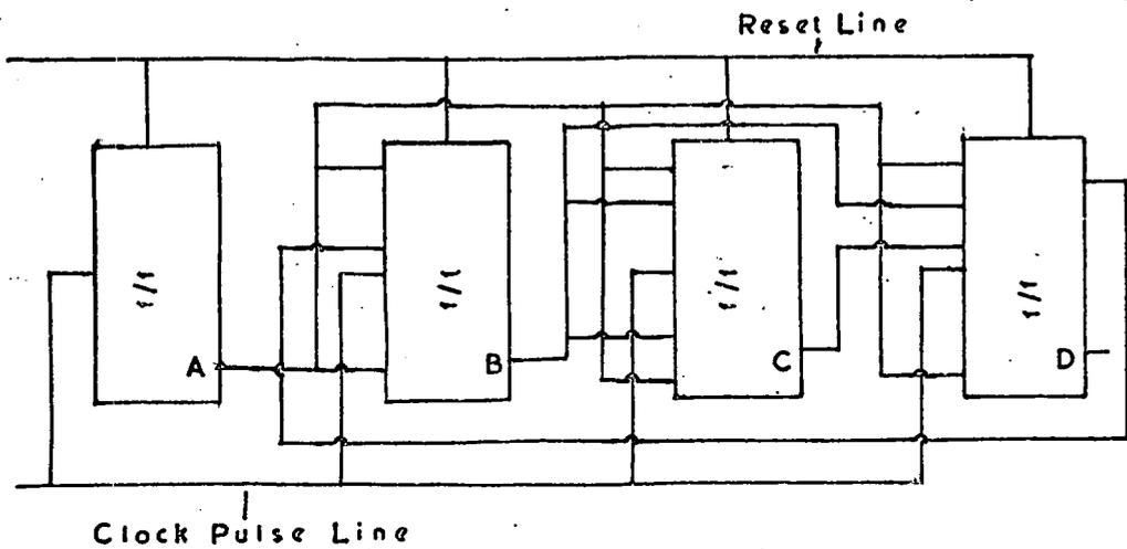
Figure A.11 The Form of a 4 Bit B.C.D. Scaler Using FCJ101 Flip-Flops.
