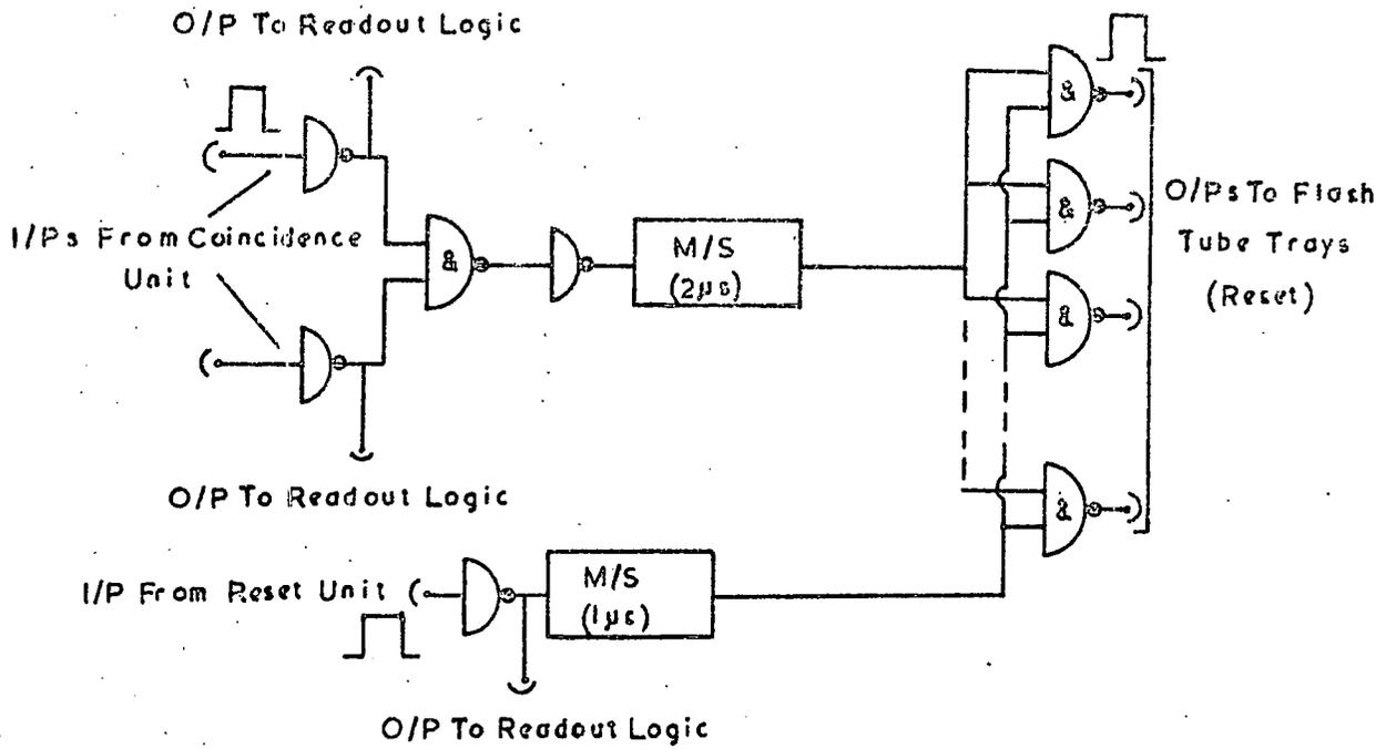
Figure 6.15. The Circuit for the Reset Logic for the Measuring and Azimuth Trays.
