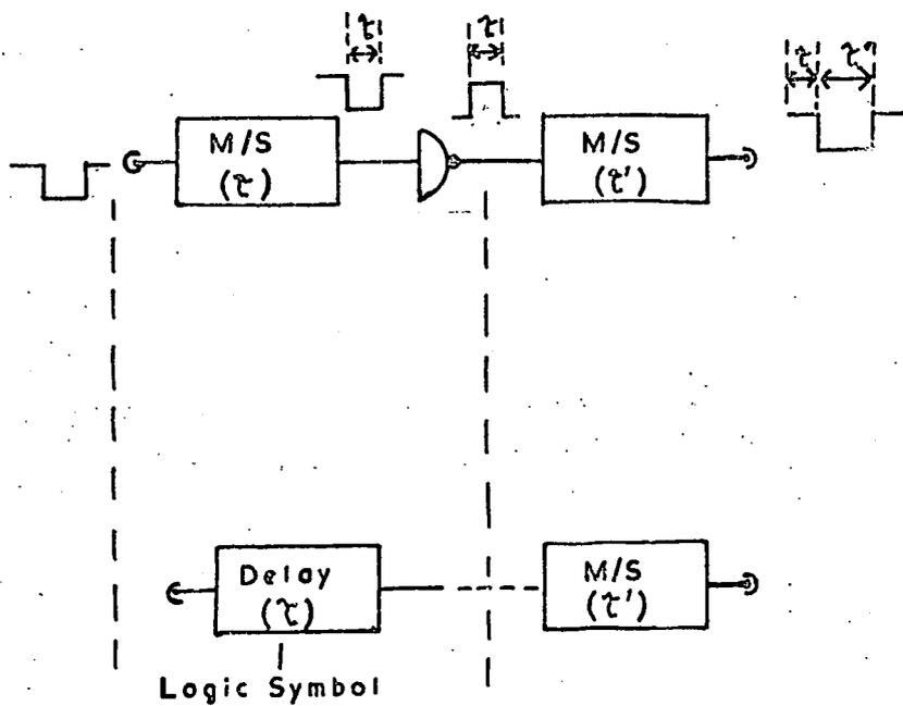
Figure A.3 The Form of the Delay Unit using Two Monostables: Connected as Shown.
