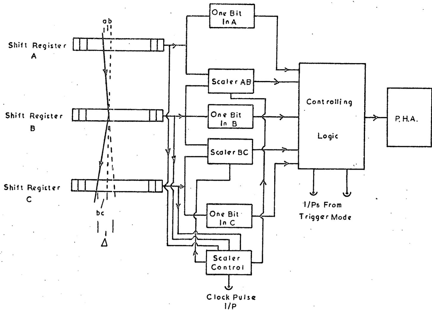
Figure 5.23 Block Diagram of the Digital Device R.U.D.I.
