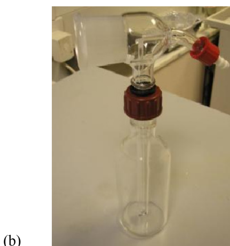
Figure 19 – (a) Diagram depicting typical experimental setup, (b) spray bottle and (c) raw graphene powder
