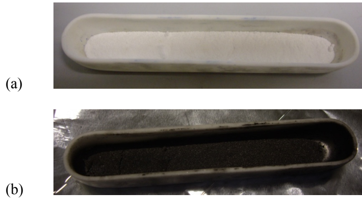
Figure A 4 – Photograph showing sodium carbonate (a) before and (b) after 1 hour in ethanol atmosphere and annealed for a further 3 hours.
