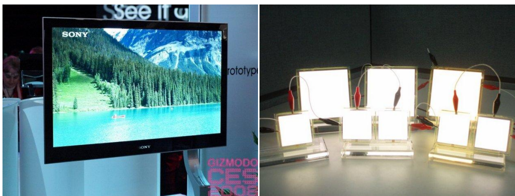
Figure 1.1: Examples of OLED display technology: Sony 27” OLED Television, and LGChem flat panel OLED lighting. Images from Refs. [4, 5], released into the public domain.
