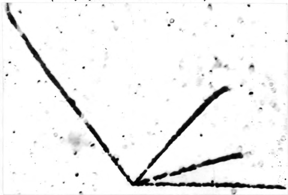
Radium Stat produced by four successive alpha-particle emissions from a single Radium nucleus. (Magnification about 2800 x)
