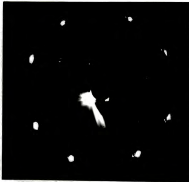
Fig. 20. Laue photograph of a strained single crystal [001] direction
