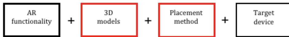
Figure 6.2: A block diagram showing the basic elements required for AR at a heritage site. Black borders are elements that could be completely “plug and play”; red borders are elements that would require special training or expertise for each individual site.
