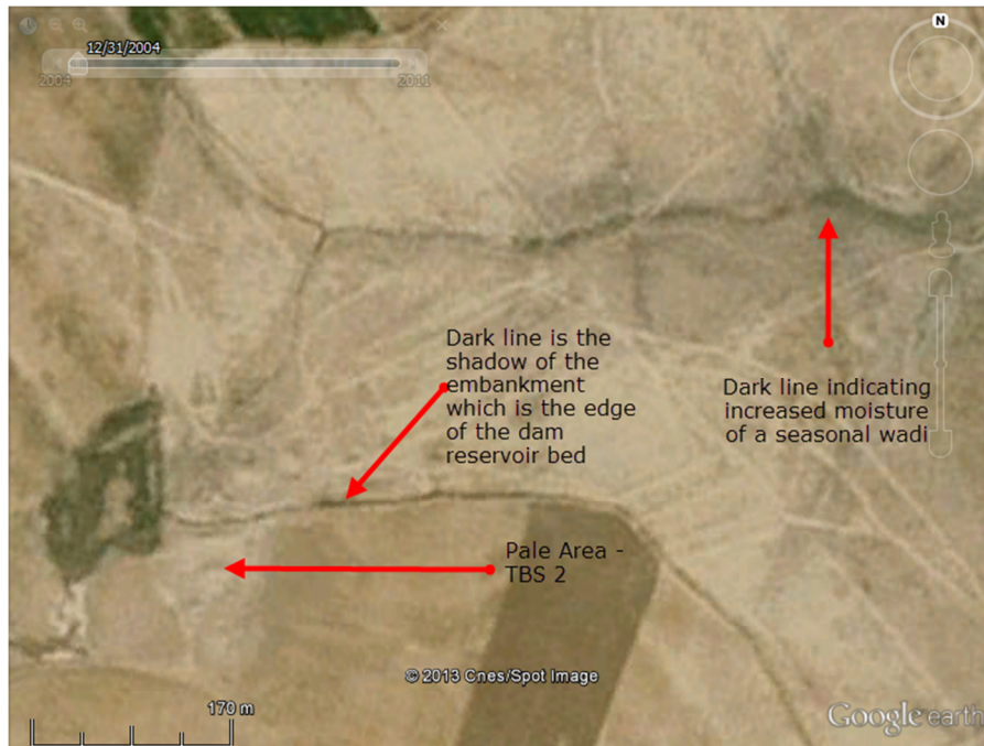
FIGURE B-15: RESERVOIR BED FOR THE WEST HASSEKE DAM BY TBS 2 ON 2004 SPOT 182
