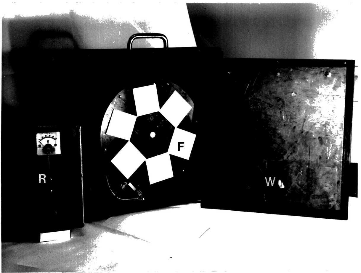
Fig.(8-1) Remote control camera for sequential synchrotron topography. Six nuclear emulsion plates, F, are mounted on a motor driven wheel. These can be rotated by operating the relay box, R, so that each plate appears sequentially behind the X-ray window W. The lead plate L prevents the beam fogging the plates.
