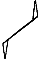
Fig 32 a. Approximate form of a failed crack. (after Brace, Paulding and Scholz, 1966)
