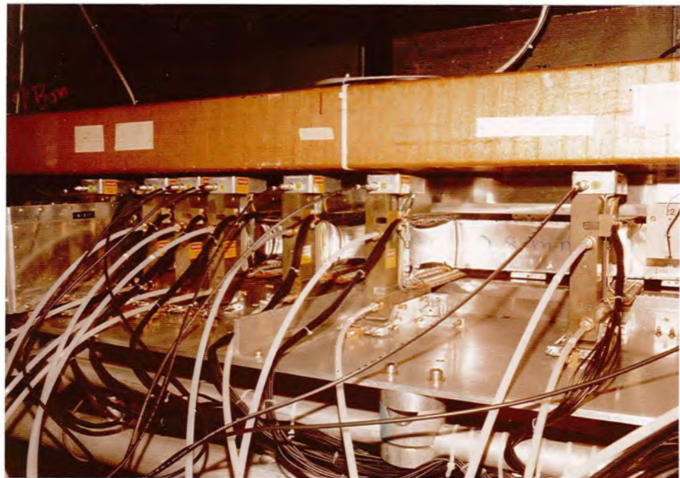
FIG 7.13(b) THE g-2 DRIFT CHAMBERS MOUNTED BETWEEN THE MAGNET POLE PIECES IN THE REGION OF THE THIN-WALLED VACUUM STORAGE TANK
