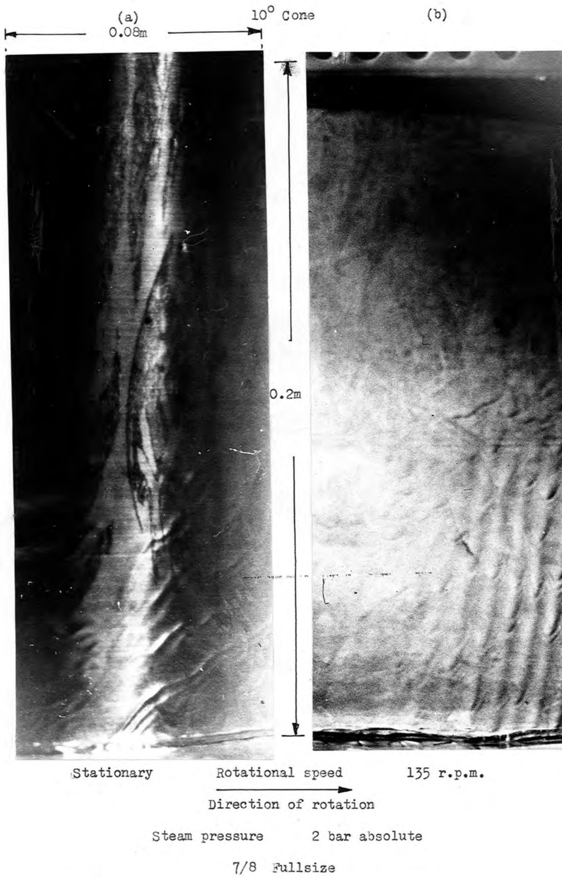
Figure 17. Variation of condensate layer profile with change of speed at constant steam pressure.
