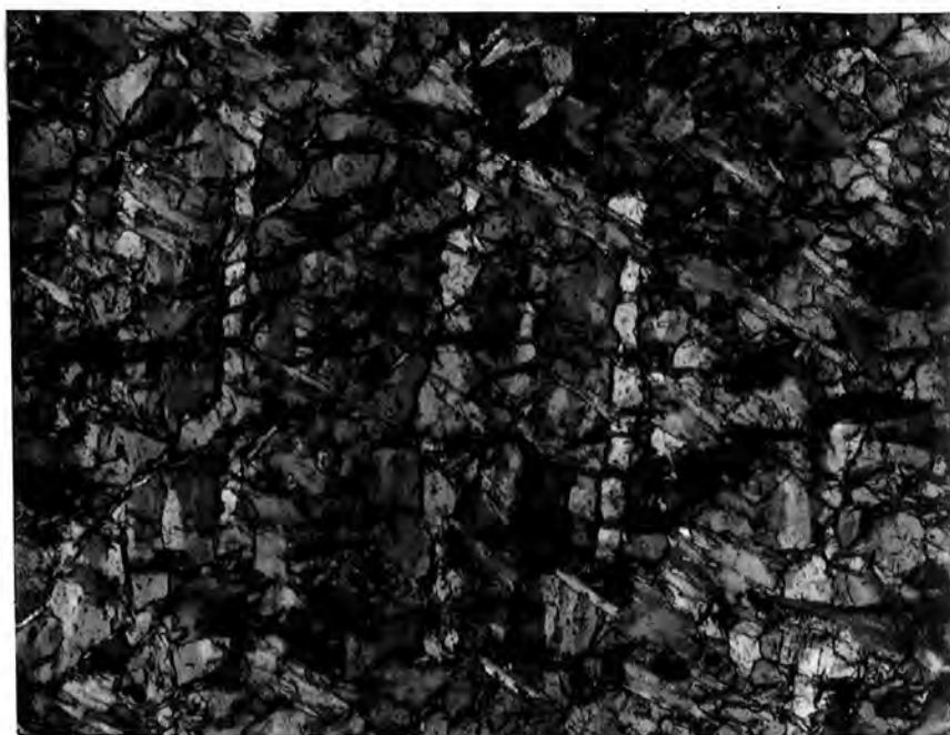
Plate 3.4 Photomicrograph: Primary olivine showing fractures parallel to original strain lamellae. Antigorite "feathers" are overprinted onto both olivine and intergranular serpentine, Sample 61615. Cross Nicols. Field width 1.7mm.
