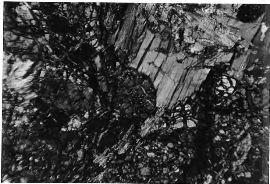
Plate 7.10 Photomicrograph: Recrystallized laths of talc and chlorite, forming a matrix to olivine (3), in Sample 60199. Light grey is talc, darker grey is chlorite. Crossed Nicols. Field width 1.7mm.
