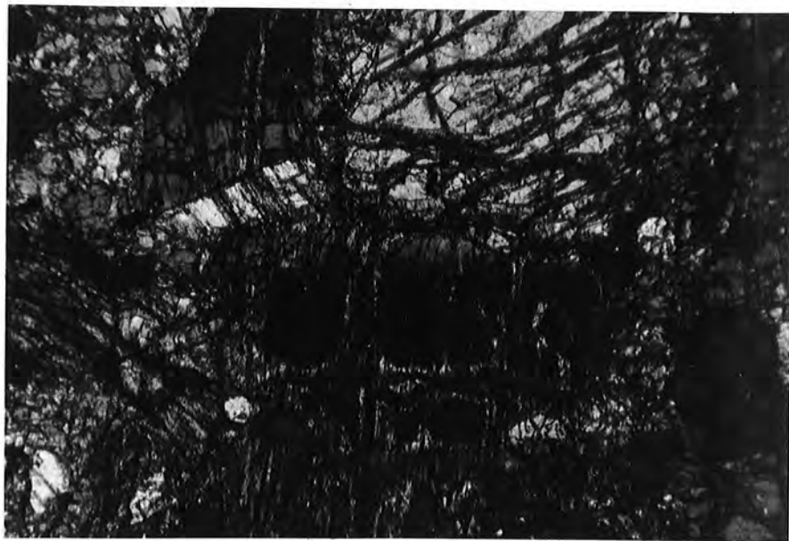
Plate 3.9 Photomicrograph: Strained, deformed, and shattered enstatite in primary peridotite, Sample 60163. Crossed Nicols. Field width 1.7mm.
