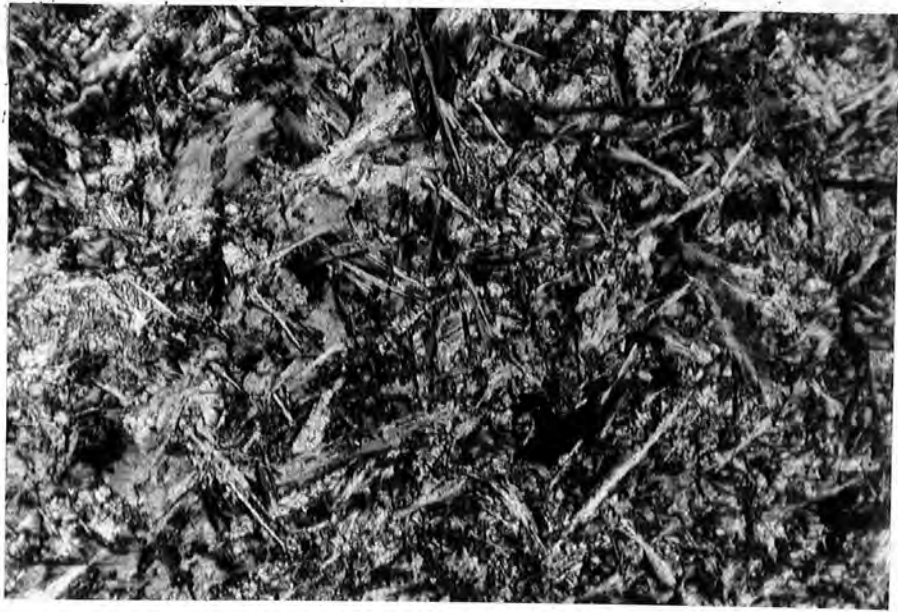
Plate 7.4 Photomicrograph: Feathery antigorite and disseminated birefringent talc, in Sample 60180. Crossed Nicols. Field width 1.7mm.
