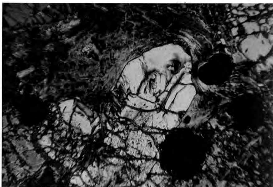
Plate 5.18 Photomicrograph: Metamorphic olivine (3), as above, with preferential marginal growth into modified matrix serpentine, Sample 61632. Crossed Nicols. Field Width 1.7mm.
