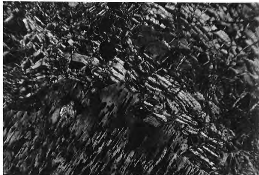
Plate 4.2 Photomicrograph: A bastite pseudomorph after enstatite in Sample 60092. Magnetite replaces diopside exsolution lamellae. The enclosing serpentinite is mesh textured. Crossed Nicols. Field width 1.7mm.
