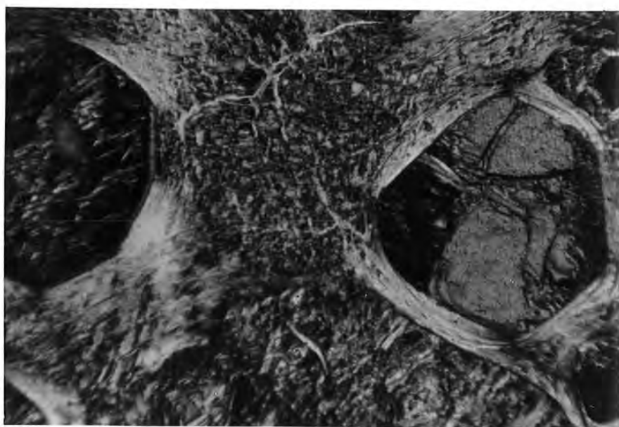
Plate 5.11 Photomicrograph: Metamorphic olivine (3) crystals in Sample 60157. Note the euhedral nature of the olivine outlines. Note also the enclosing modified matrix serpentine. Crossed Nicols. Field width 1.7mm.
