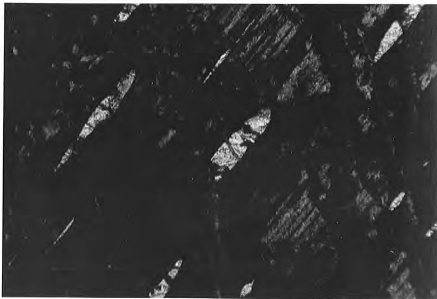
Plate 3.10 Photomicrograph: Relict diopside exsolution blebs in a bastite pseudomorph in Sample 60067. Crossed Nicols. Field width 1.7mm.
