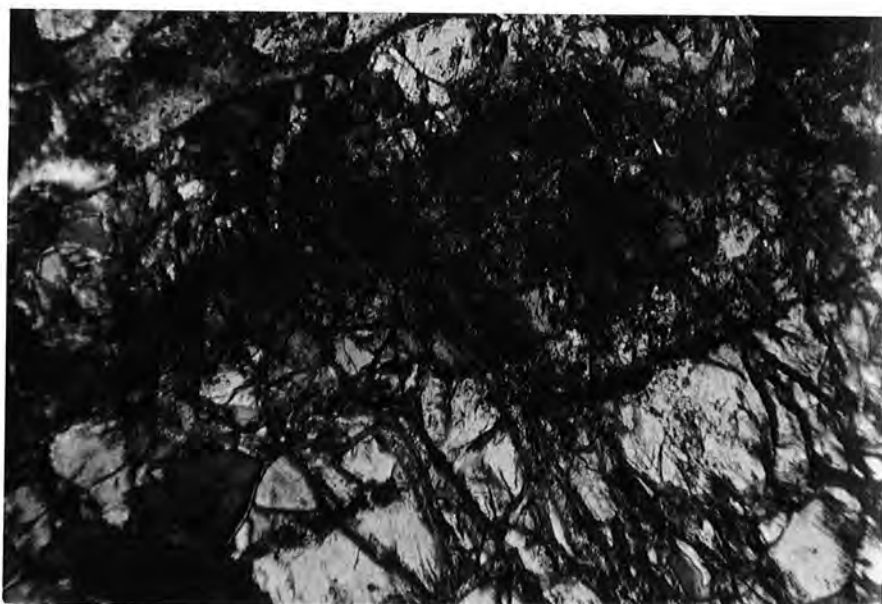
Plate 5.22 Photomicrograph: Recrystallized asbestos in Sample 61525. Note the magnetite partition inherited from asbestos. Crossed Nicols. Field width 1.7mm.
