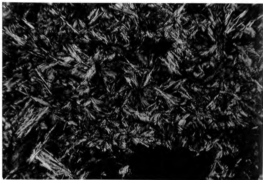
Plate 7.3 Photomicrograph: Feathery, antigorite replacing metamorphic olivine, in Sample 60107. Crossed Nicols. Field width 1.7mm.
