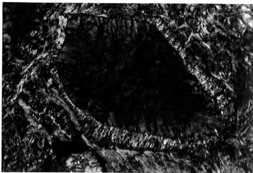
Plate 7.6 Photomicrograph: A serpentine pseudomorph after olivine (3), in Sample 60102. The interface between modified matrix serpentine and retrogressive serpentine is enriched with brucite and magnetite. Crossed Nicols. Field width 1.7mm.
