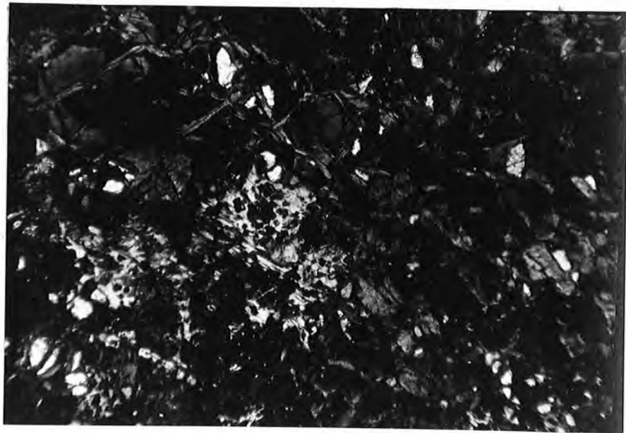
Plate 7.8 Photomicrograph: Granular spinel (4) cubes in recrystallized chlorite, Sample 61603. Crossed Nicols. Field width 1.7mm.
