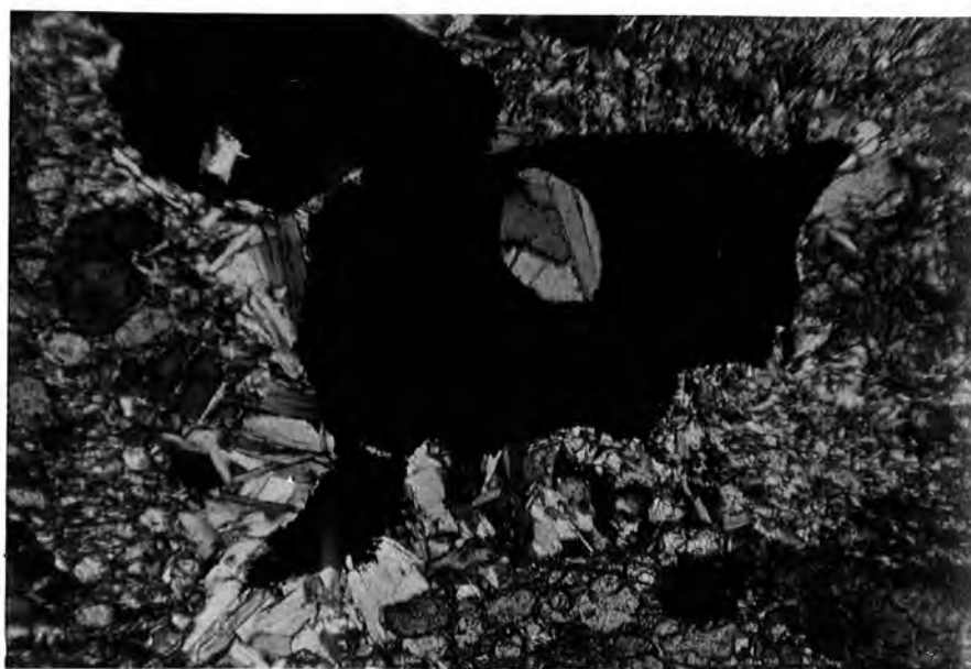
Plate 5.10 Photomicrograph: Recrystallized chlorite enveloping an altered poikilic spinel, in Sample 60341. The halo is analogous to the Al-serpentine envelope shown in Plate 5.6. Crossed Nicols. Field width 1.7mm.
