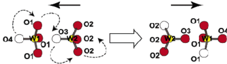
Figure 4-2 Oxygen mobility mechanism responsible for the \alpha to \beta -phase transition in cubic ZrW_2O_8 . (5)
