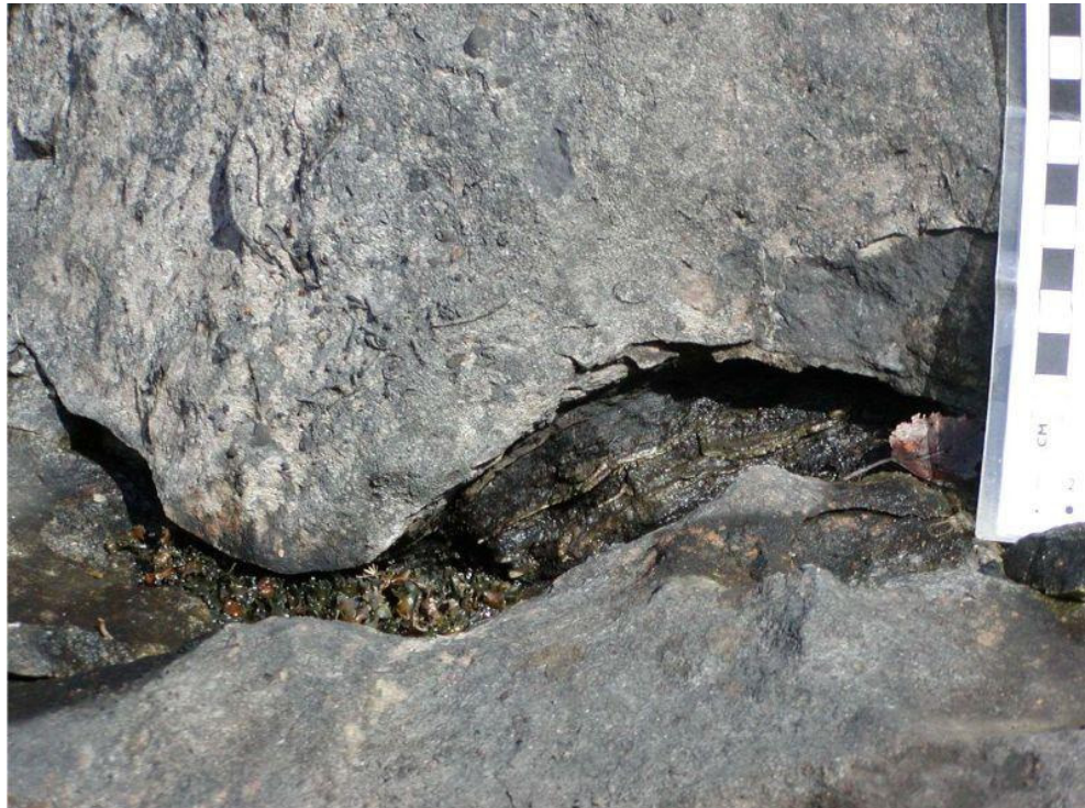
Figure 3.23. Undulating mudstone parting. Note thin calcareous units within bedding plane. Bedding plane approximately 20 millimetres thick. (Lanehead Quarry Weardale OS 39885 54052)
