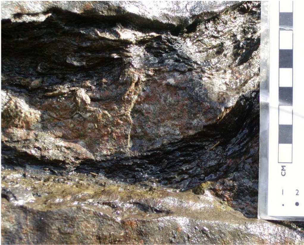
Figure 3.24. Undulating mudstone parting. Bedding plane varying between 10 millimetres and 30 millimetres thick. (Lanehead Quarry Weardale OS 39885 54052)
