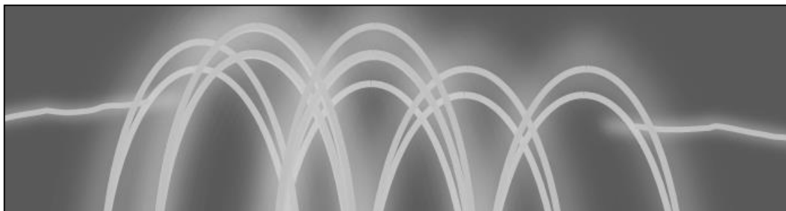
Figure 3.22: Depiction of scatter on a z-scope image, where parabolas cause subjectivity in inferring the bed trace
