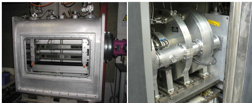
Figure 3.5. Photographs of (a) the frame overlap mirror and (b) the choppers in the FIGARO instrument
