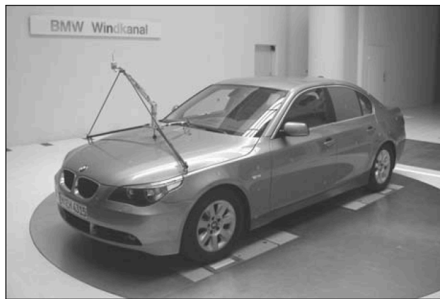
Figure 1.33: Probe mounted ahead of windscreen, from Mayer et al. (2007)
