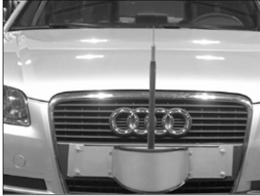
Figure 1.36: Front-mounted probe, from Lindener et al. (2007)
