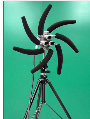
(b) Portable array, from HEAD Acoustics NVH Division (2010)
