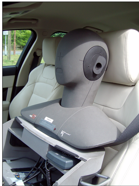
Figure 2.12: Acoustic head installed in front passenger seat
