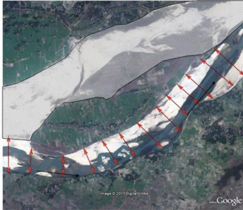
Figure 3.9 Representation of an island in the Damodar River within LISFLOOD-FP. Red arrows show the 1D configuration of the main channel. The shallower secondary channel and the floodplain, depicted with shading, are handled by the 2D component of the model.
