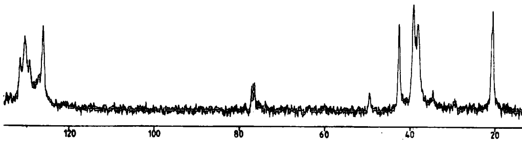
Figure 3.19. ^{13}\text{C} N.m.r. spectra for Compound (XXIII) and derived polymer
