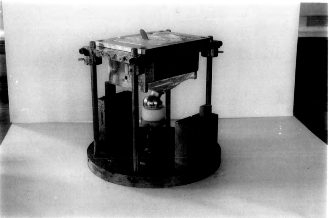
Figure 4.16 Setting-up jig using base with central cup for positioning femoral head
