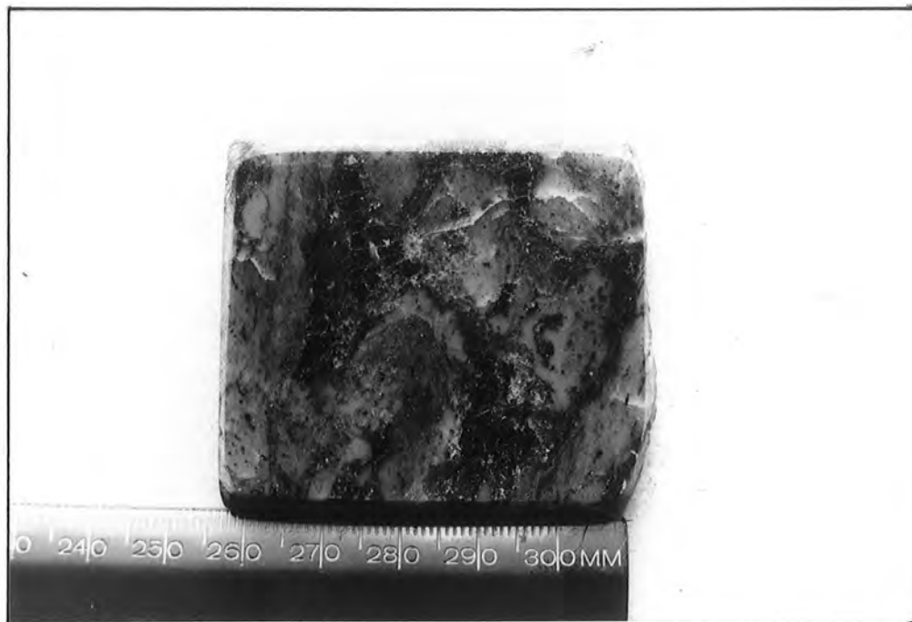
Plate 40. F_1 fold in quartz+sphalerite layer from the W locality.
