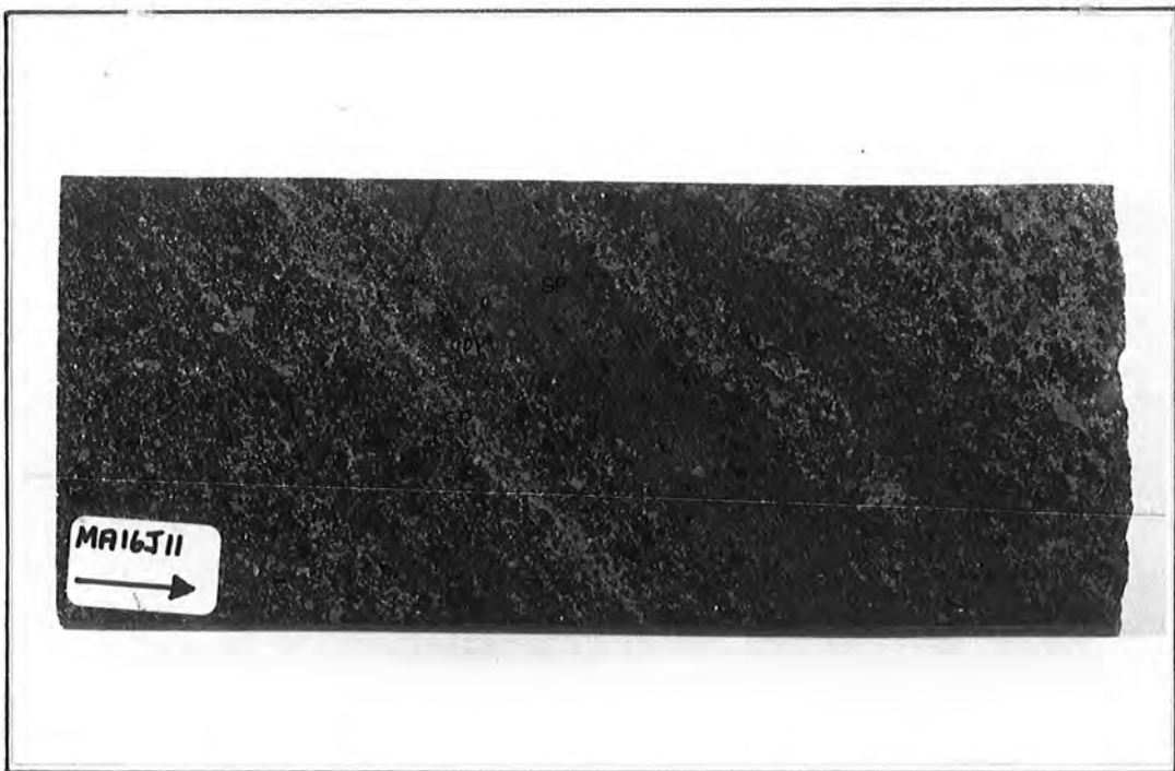
Plate 33. Banded massive sulphides, J massive sulphide deposit. Py - pyrite; sp - sphalerite; cp - chalcopryrite; po - pyrrhotite. Natural size.
