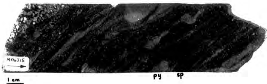
Plate 47. Banded pyrite+sphalerite ore. Possible slump structures, pyrite balls and concretions.
