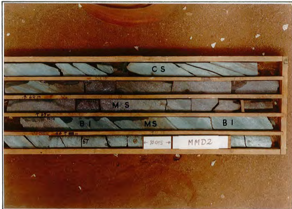
Plate 37. Massive sulphide intersection from hole MMD2 D locality. Cs- chlorite schist with sphalerite bands (brown); MS - massive sulphide, mainly sphalerite; BI - basic intrusive.
