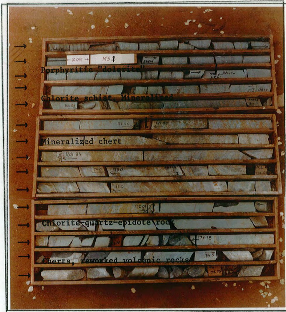
Plate 35. Sulphide intersection from hole MS1, MGZ locality. Massiv sulphide unit is absent. New points from base to top of each run.
