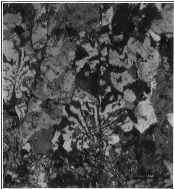
Plate 27. Granophyric texture in quartz diorite phase of the Rooiwater Igneous Complex. Sample CD21, crossed polars.
