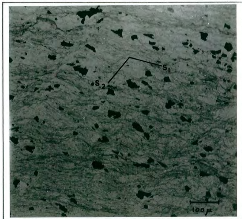
Plate 11. S_1 and S_2 in thin section. Micaceous schists, Transition Zone sequence. Sample MA28W2. Plane polarised light.
