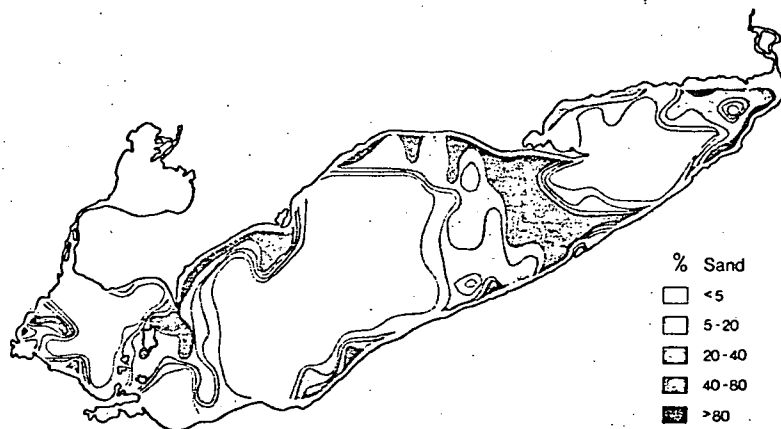
Distribution of percent sand-size fraction in the surficial sediment of Lake Erie.
