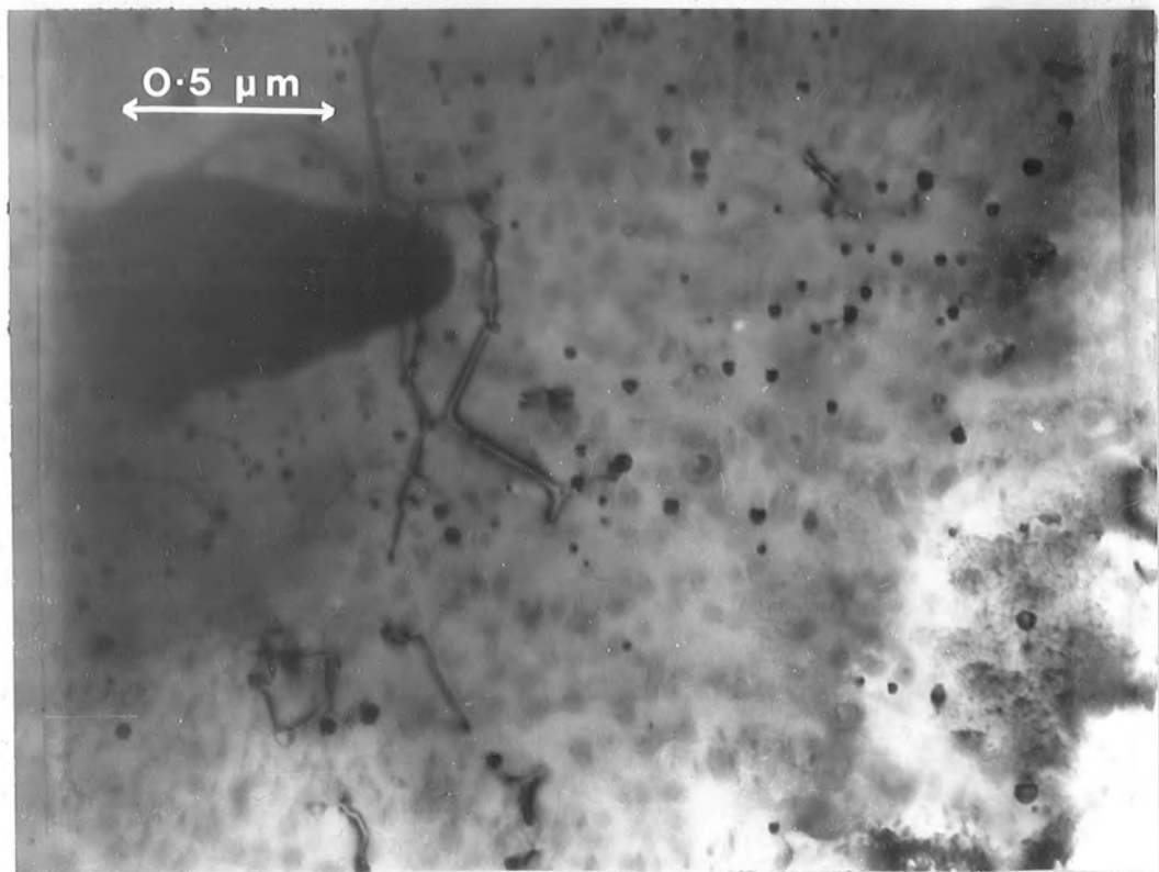
Fig. 7.21(c) The same as in figure 7.21(a) from another region showing Precipitates and Decorated Dislocations.
