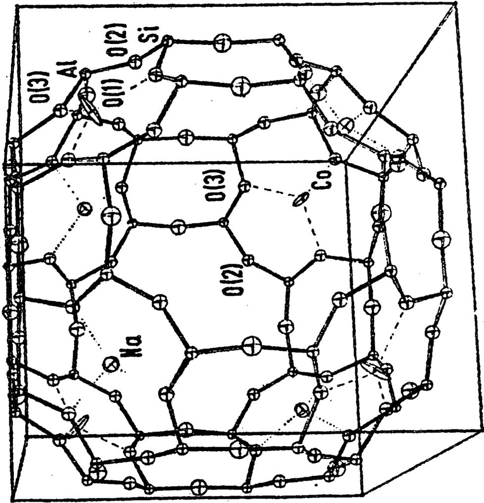
Fig.3 Co-A zeolite fully dehydrated
