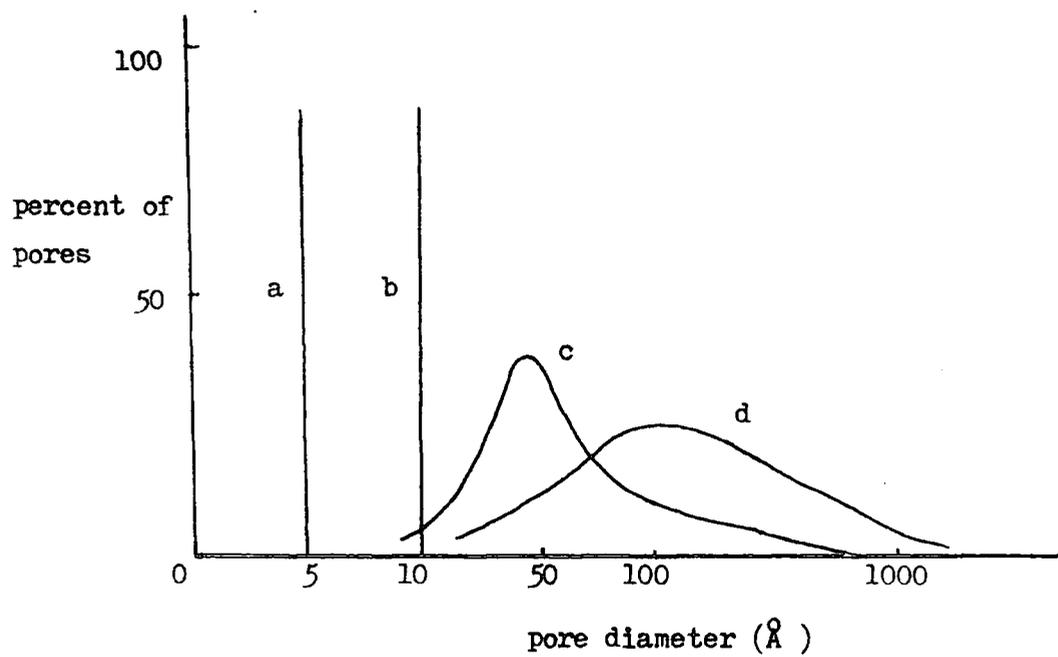
Fig.3 pore size distribution of various molecular sieves
