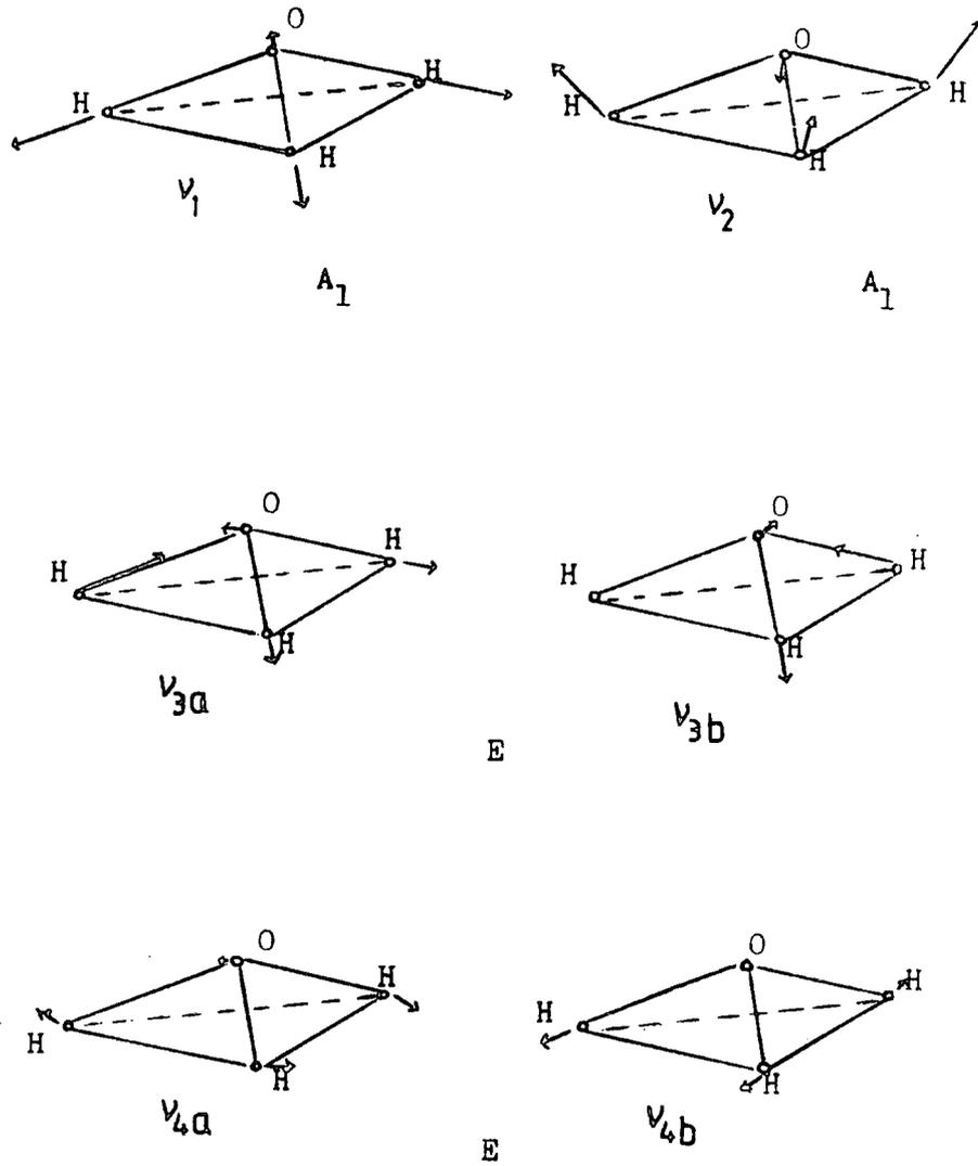
Fig.12 Normal modes of vibration for  $H_3O^+$  (30)
