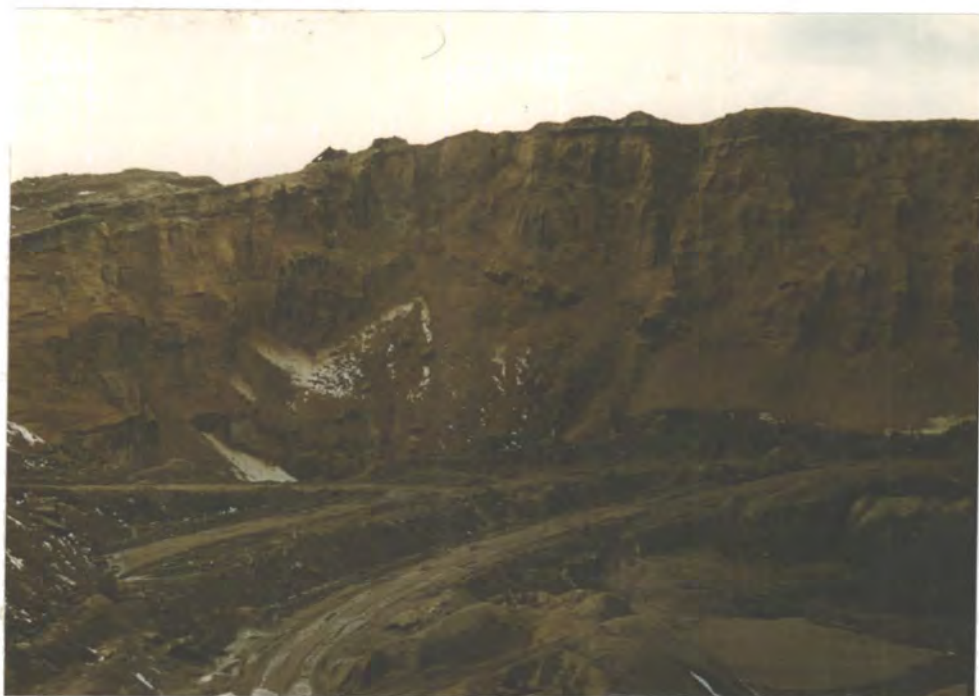
FIG. 5.14 View of the west face of Sherburn Hill Sand Pit. The top of the face corresponds closely to the top of the Yellow Sands. Distance from the top of the face to the floor of the quarry \sim 30\text{m} .
