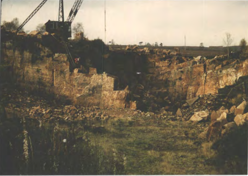
FIG. 9.2 Halfwaywell Quarry (NY 533352), the only active quarry in the Penrith Sandstone. The quarry is excavated in a single, well-cemented, trough-shaped set directed towards 310^{\circ} .
