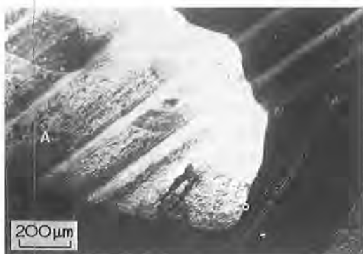
Figure 6 Secondary emission micrograph of the region shown in Fig. 2 where -3\text{ V} is applied to grain A.
