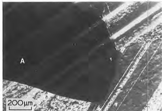
Figure 5 Secondary emission micrograph of the region shown in Fig. 2 where +3 V is applied to grain A.
