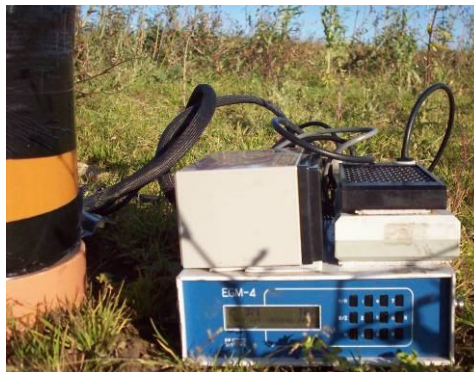
Figure 4.3 IRGA used to measure CO 2 flux from/to the atmosphere
