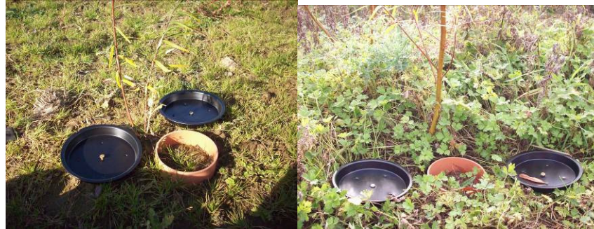
Figure 8.5 Litter trays to measure carbon accumulated in leaf litter
