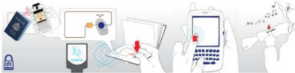
Figure 1. : A depiction of several electronic switch and pressure sensing applications of Quantum Tunnelling Composite™.
