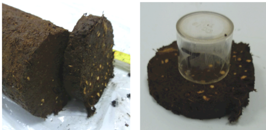
Figure 3.13 Sediment cores were cut into individual 0.01 m slices before using the cutter to remove a section of known volume to calculate bulk density.
