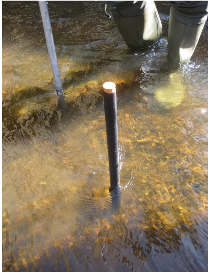
Figure 3.5. Equipment installed in the riverbed to sample from the hyporheic zone.
