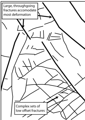
Figure 5.4b. Multiple fracture sets exposed on the wave-cut platform at Praia das Focas show larger, throughgoing NW-SE fractures, with smaller fractures between them. Many of these fractures may be joints, formed either during tectonics or uplift. Identification of offset is impossible, though some of these fractures do show slickenlines.
