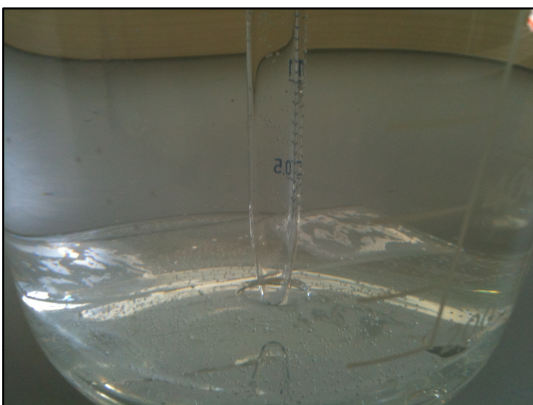
B Figure 3.2 A) Image of several of diatom absolute abundance apparatus running simultaneously. B) Close-up image of coverslips at bottom of beaker, with the pipette through the central hole of an inverted petri dish.
