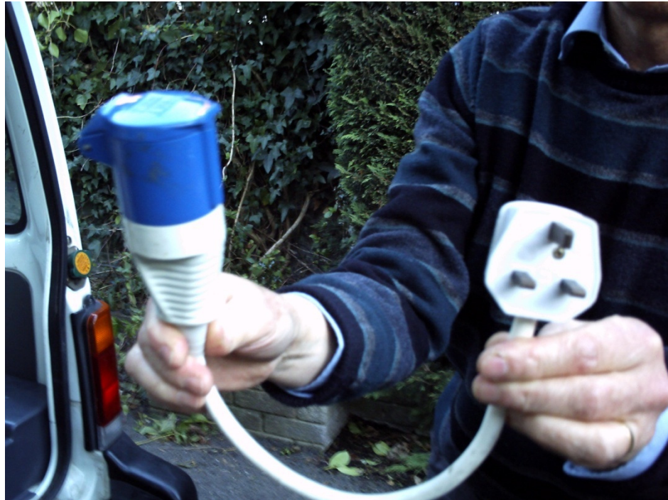
Fig 6.2 - A driver displays a 16-amp to 13-amp adapter. Most drivers in the study carry this simple piece of kit at all times.
