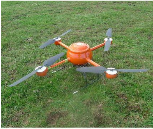
Figure 5.2a: Microdrone MD4-200 helicopter.
