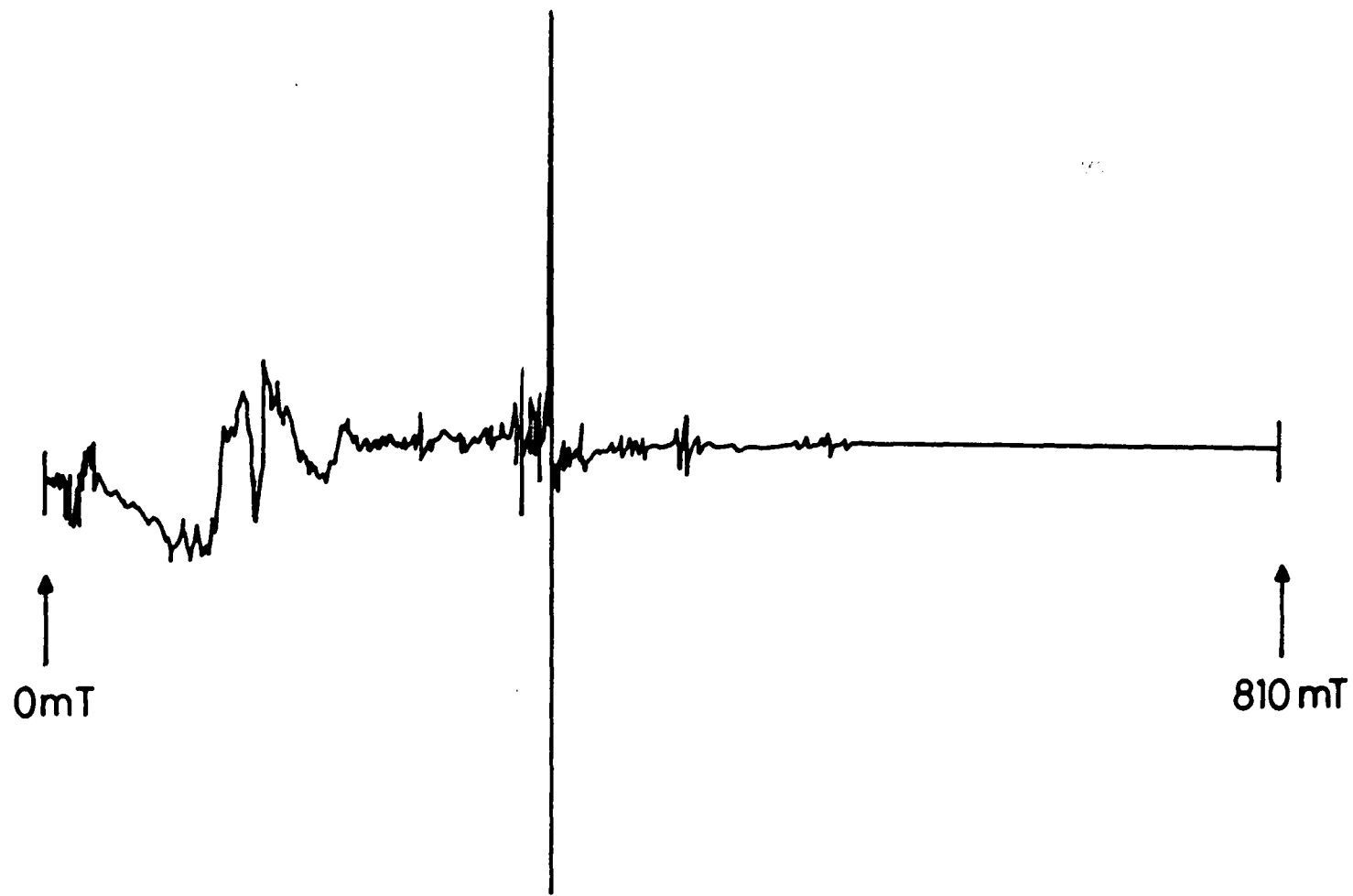
FIGURE 7.12 EXTENDED E.P.R. SPECTRUM OF SINGLE CRYSTAL Cr/MgO; 15,100 p.p.m. Cr, 293K, H// <100>, \nu = 9.2540 GHz.
