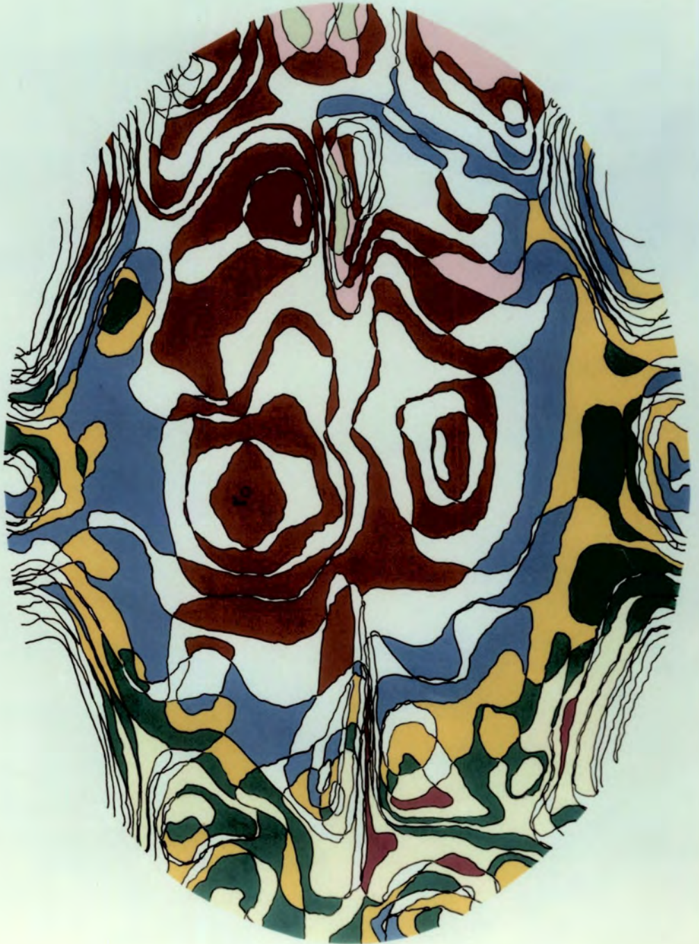
Fig. 3.12: Relative lattice strain map of the Wacker low pressure GaAs sample. All values are relative to position r_0
