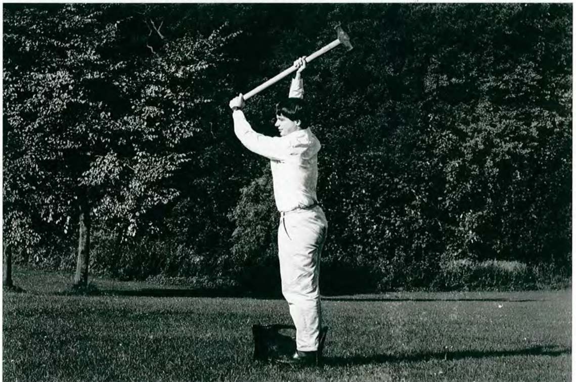
Plate 4 S wave source Shear wave stand with operator
