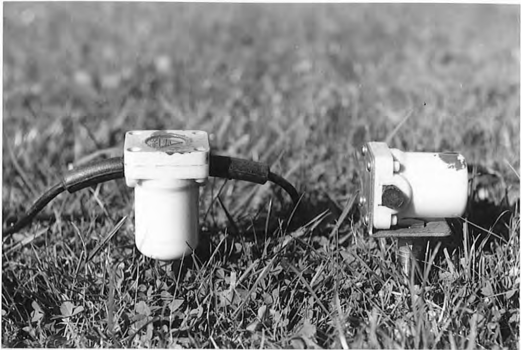
Plate 5 Receivers Vertically and horizontally mounted geophones
