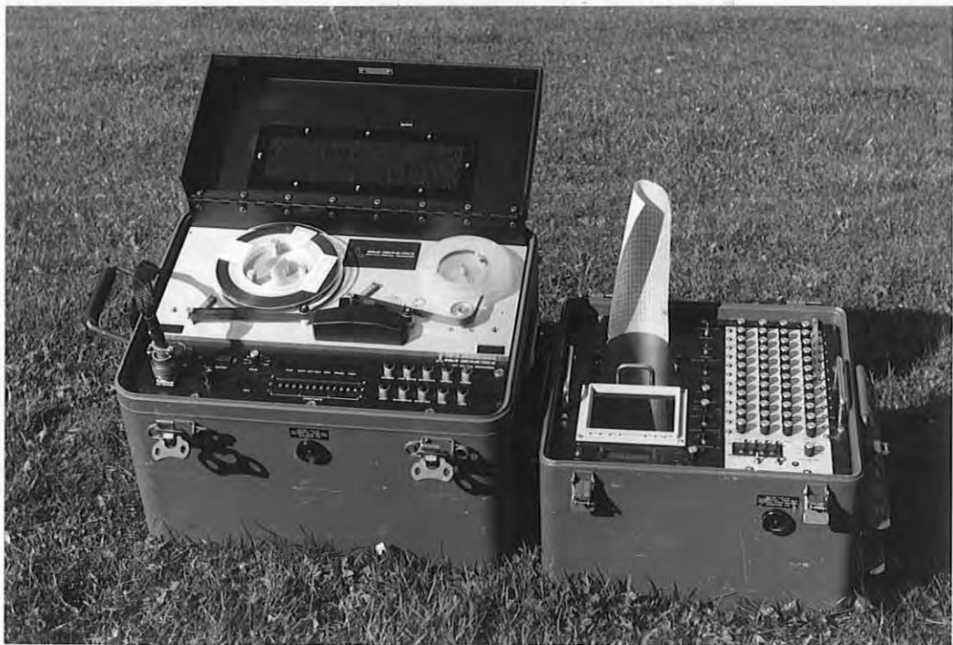
Plate 6 Recording system Nimbus ES-1210F enhancement seismograph with EG&G DMT-911 digital tape recorder
