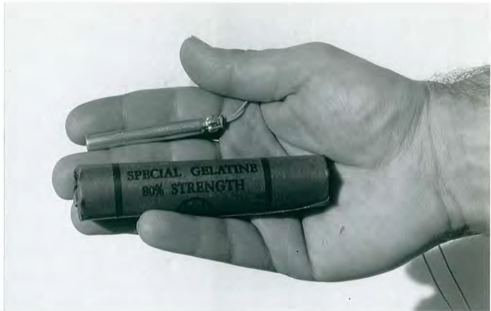
Plate 3 P wave source Seismic detonator and 2oz stick of gelignite
