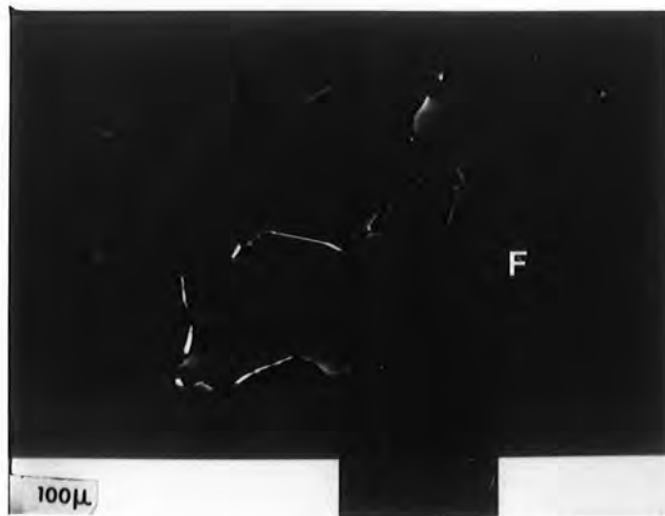
EBIC image recorded at zero bias
