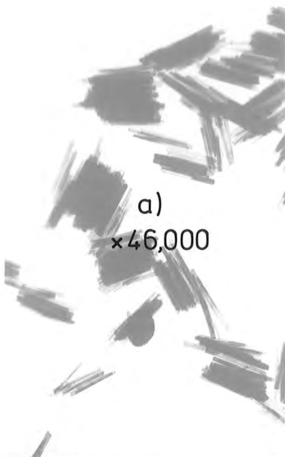
Fig.8.1 Electron micrographs of some hydrated iron(III) oxide species: a) \beta -FeOOH, b) \alpha -FeOOH.1, c) \alpha -FeOOH.2
